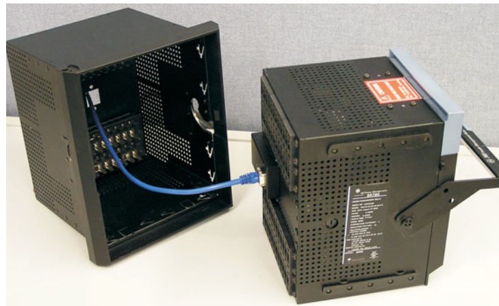
Figure 3-8: Ethernet Cable Connection
