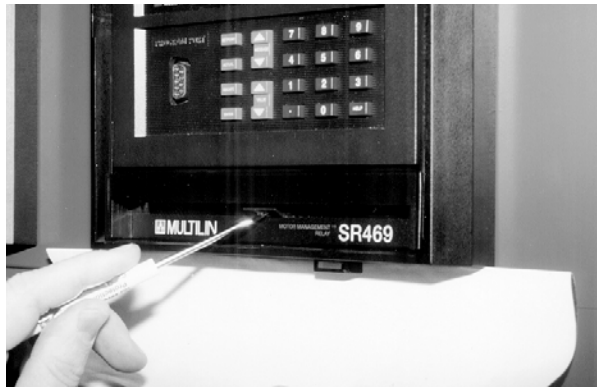
Figure 2-6: PRESS LATCH TO DISENGAGE HANDLE
