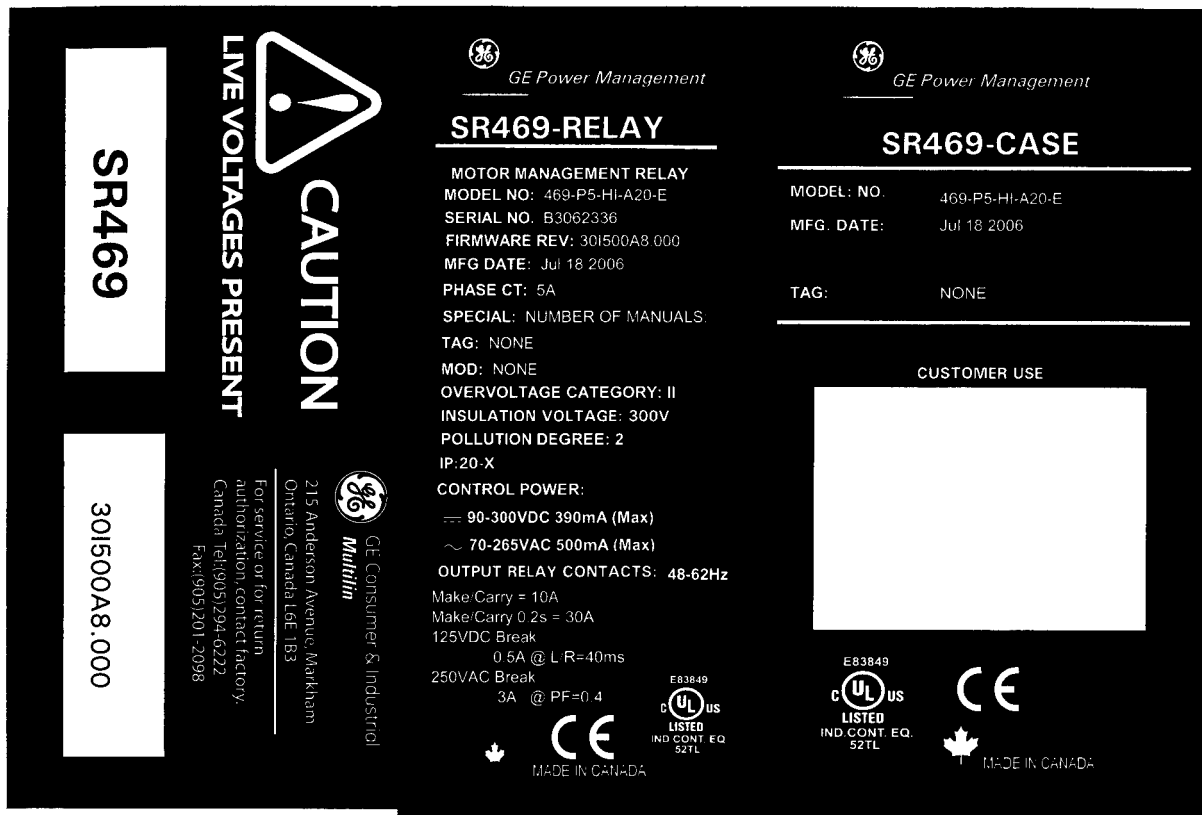
Figure 2-3: CASE AND UNIT IDENTIFICATION LABELS
