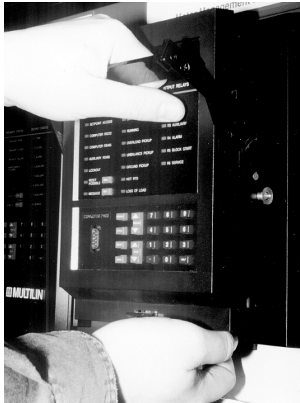
Figure 2–8: SLIDE UNIT OUT OF CASE
