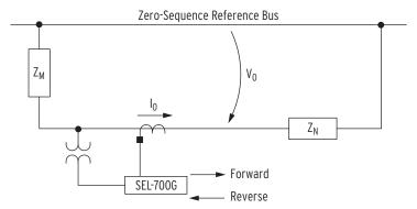
Figure 4.91 Zero-Sequence Impedance Network and Relay Polarity
