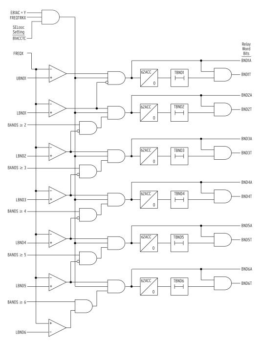
Figure 4.45 Abnormal Frequency Protection Logic Diagram
