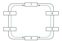
Figure 7.16 Physical Ring Without Loop Mitigation
