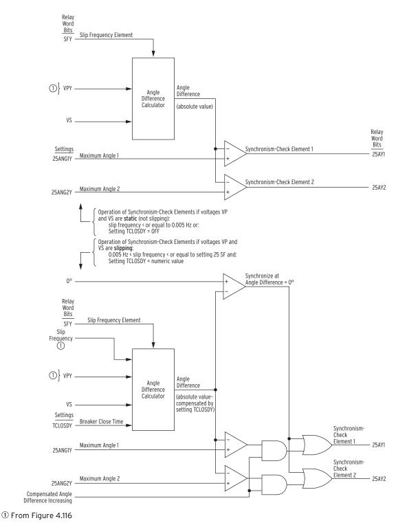
Figure 4.117 Synchronism-Check Elements
