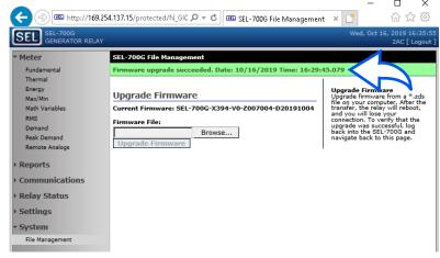
Step 5. Check that the relay firmware version matches the version that was used for the upgrade and that the relay is enabled.
