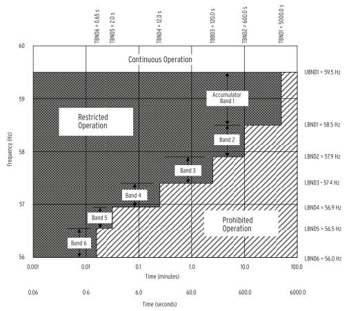
Figure 4.44 Example Turbine Operating Limitations During Abnormal Frequency
