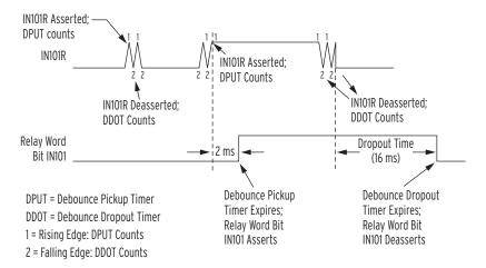
Figure 4.155 Timing Diagram for Debounce Timer Operation When Operating in AC Mode
