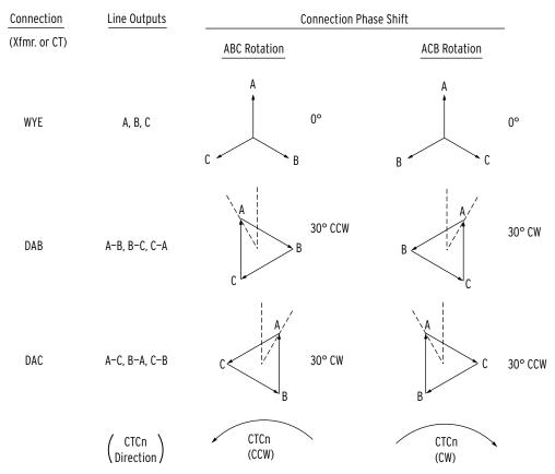
Figure 4.13 Winding Connections, Phase Shifts, and Compensation Direction
