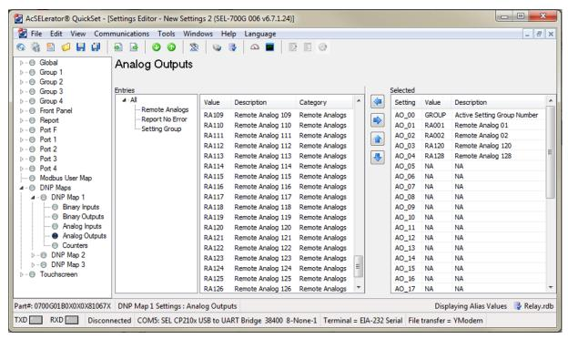
Figure D.9 Analog Output Map Entry in QuickSet
