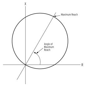
Figure 4.25 Phase-to-Phase Distance Element Operating Characteristics
