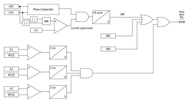
Figure 4.11 High Security Mode RESET Logic
