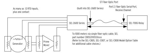
Figure 2.33 Generator Thermal Protection With an SEL-2600 RTD Module and an SEL-700G
