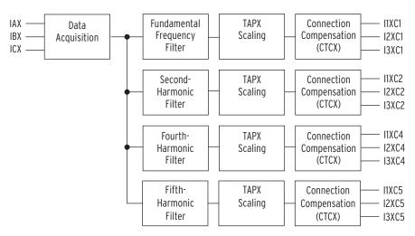
Figure 4.3 Winding X Compensated Currents
