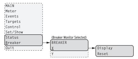
Figure 8.24 MAIN Menu and BREAKER Submenu
