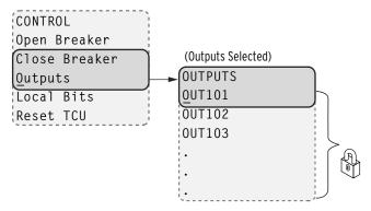
Figure 8.19 CONTROL Menu and OUTPUTS Submenu
