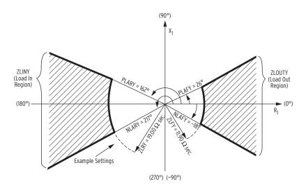
1 To Figure 4.87 Figure 4.95 Load-Encroachment Logic for Y Side
