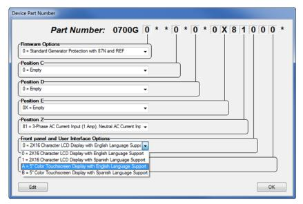
Figure 9.13 Device Part Number Touchscreen Configuration Option
