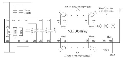
Figure 2.14 Control I/O Connections-4 AI/4 AO Option in Slot D
