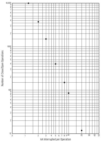
Figure 5.18 Plotted Breaker Maintenance Points for a 25 kV Circuit Breaker
