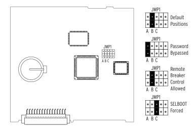
Figure 2.7 Pins for Password, Breaker Control, and SELBOOT Jumper
