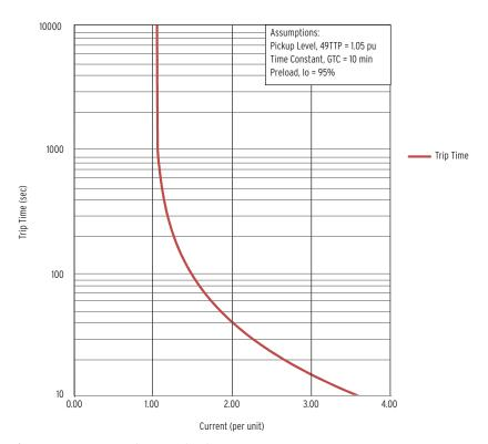
Figure 4.37 Generator Overload Curve
