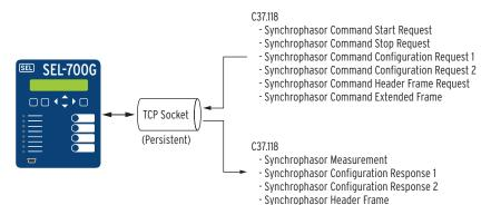
Figure K.4 TCP Connection
