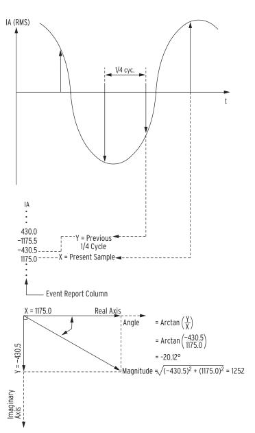
NOTE: The arctan function of many calculators and computing programs does not return the correct angle for the second and third quadrants (when X is negative). When in doubt, graph the X and Y quantities to confirm that your calculator reports the correct angle.
