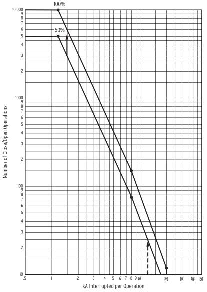
Figure 5.24 Breaker Monitor Accumulates 100 Percent Wear
