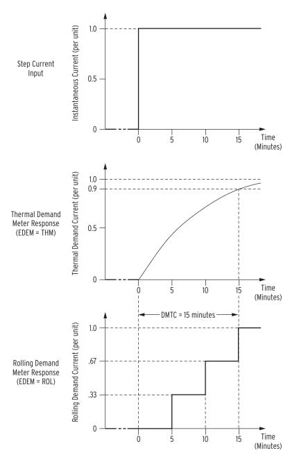
Figure 4.130 Response of Thermal and Rolling Demand Meters to a Step Input (Setting DMTC = 15 minutes)
