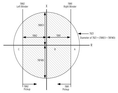
Figure 4.46 Single-Blinder Scheme Operating Characteristics
