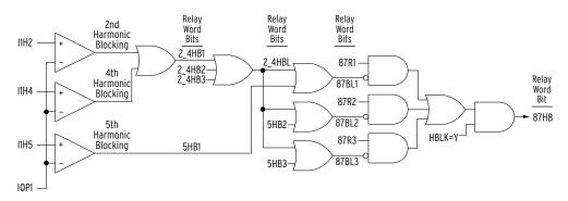
Figure 4.6 Differential Element Harmonic Blocking Logic
