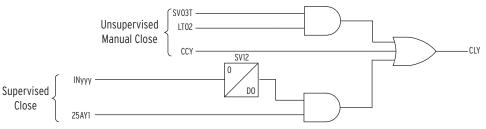
Figure 4.139 Typical Generator or Intertie Close CL Logic (SEL-700G or GT)
