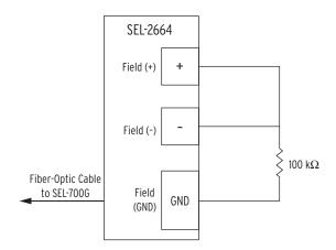
Figure 11.5 Verifying the Connection Between the SEL-2664 and the **SEL-700G**
