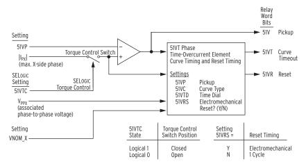
Figure 4.29 Voltage-Restrained Phase Time-Overcurrent Element 51VT
