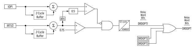
Figure 4.9 Delta IRTn and Delta IOPn External Event Detector Logic
