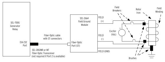
Figure 2.34 Field Ground Protection With an SEL-700G Relay
