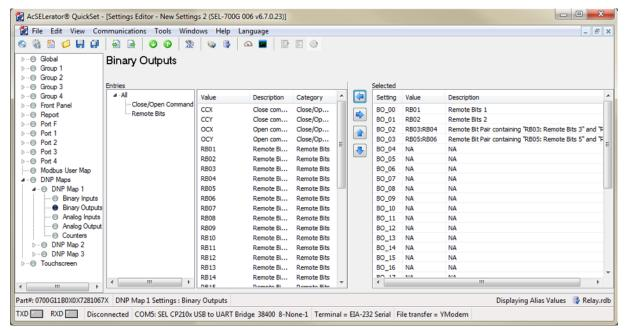
Figure D.11 Binary Output Map Entry in QuickSet
