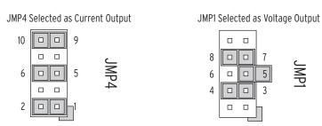
Figure 2.5 Current Output Jumpers Figure 2.6 Voltage Output Jumpers
