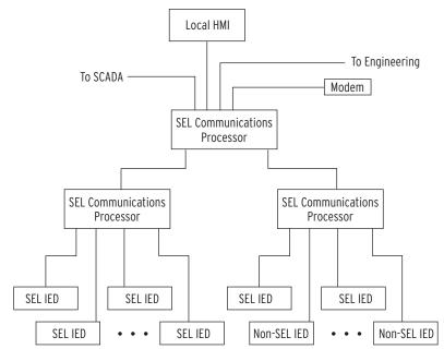
Figure C.2 Multitiered SEL Communications Processor Architecture
