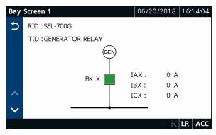
Figure 9.5 Bay Screens Application Display With a Single-Line Diagram
