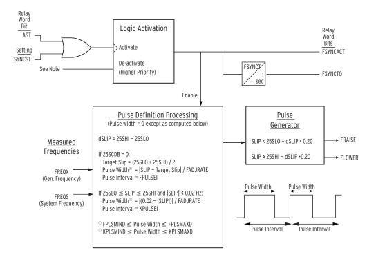
Note: The logic is enabled when settings E25X := YES and EAUTO := DIG. The logic is de-activated and disabled when any of the following is true:
