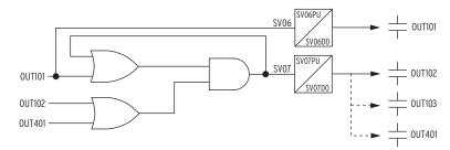
Figure 4.145 Example Use of SELogic Variables/Timers
