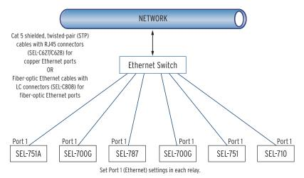
Figure 7.1 Simple Ethernet Network Configuration
