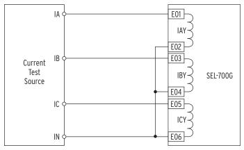
Figure 11.7 CTRY Current Source Connections
