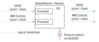
Figure G.11 Relay Operations in Blocked Mode
