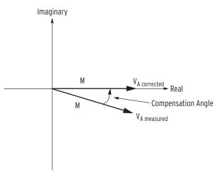
Figure K.3 Correction of Measured Phase Angle
