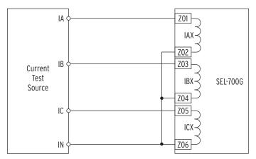
Figure 11.6 CTRX Current Source Connections
