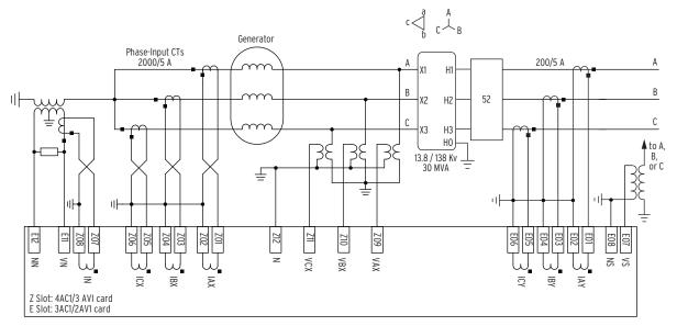
Figure 2.23 SEL-700G1+ Relay AC Connection Example-High-Impedance Grounded Generator With Step-Up Transformer Included in Differential Zone (With Synchronism Check and 100% Stator Ground Protection)
