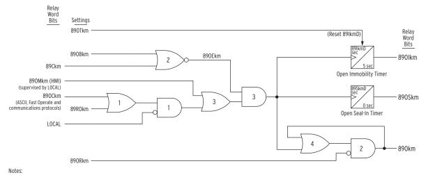
k = 2P, 3PL, or 3PE m = switch number (1-8 if k = 2P; 1-2 if k = 3PL or 3PE) Each three-posotion disconnect (3P) is a combination of one in-line and one earthing disconnect (e.g., 3PL1 and 3PE1).
