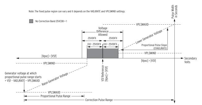
Figure 4.123 Voltage Connection Characteristics When GENV+ = N
