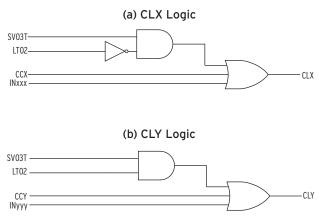
Figure 4.140 Typical Feeder Close CL Logic (SEL-700GW)
