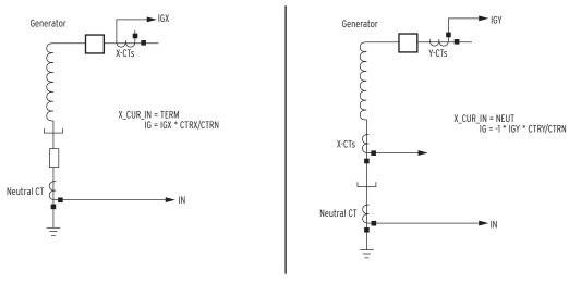
Figure 4.15 Effect of X\_CUR\_IN Setting on Residual Current (IG)
