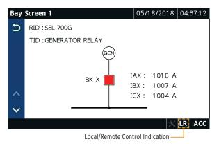
Figure 9.4 Local/Remote Control Mode Indication
