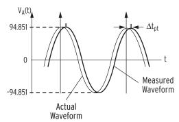
Figure K.2 Waveform at Relay Terminals May Have a Phase Shift
