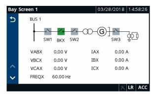
Figure 9.24 IEC SEL-700G1 With GSU and Disconnects
