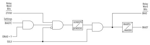
Figure 4.52 Inadvertent Energization Logic Diagram
