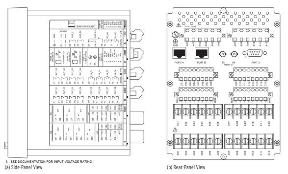
Figure 2.9 SEL-700GT+ With Dual Copper Ethernet, 4 DI/4 DO, 8 DO, 3 ACI/4 AVI, 4 ACI/3 AVI (Relay MOT 0700GT1A1A2X75850630)
