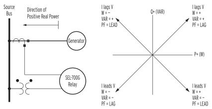
Figure 5.1 Complex Power Measurement Conventions
