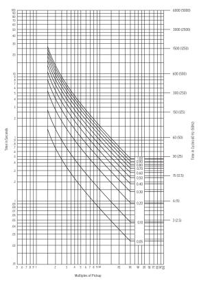
Figure 4.68 IEC Class B Curve (Very Inverse): C2
