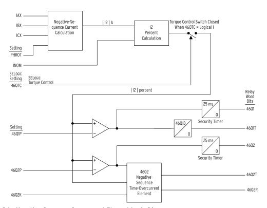
Figure 4.34 Negative-Sequence Overcurrent Element Logic Diagram
