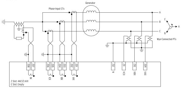
Figure 2.20 SEL-700GO Relay AC Connection Example-High-Impedance Grounded Generator Without Current Differential Protection
