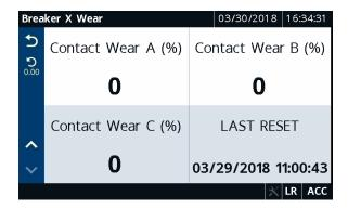
Figure 8.40 Breaker Wear A, B, C, and Last Reset
