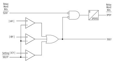
Figure 4.133 Pole Open Logic Diagram, Breaker 52Y
