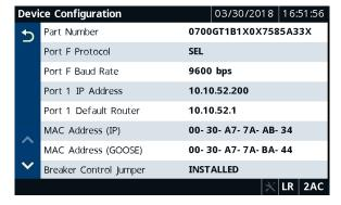
Figure 8.65 Device Configuration
