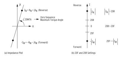
Figure 4.92 Zero-Sequence Impedance Plot for Solidly-Grounded, Mostly Inductive System
