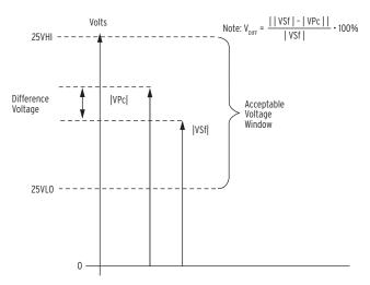
Figure 4.110 Synchronism-Check Function Voltage Element Characteristic
