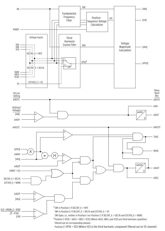
Figure 4.22 64G Logic Diagram
