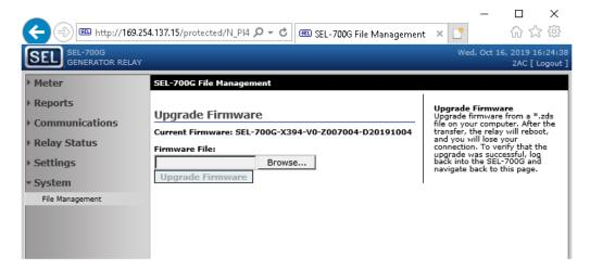
Figure 3.14 Upgrade Relay Firmware From the File Management Webpage
