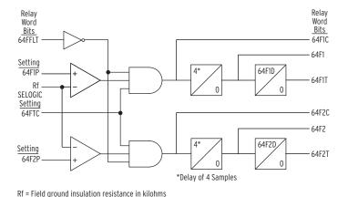
Figure 4.23 Field Ground Protection (64F) Elements Logic
