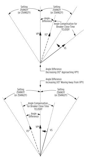
Figure 4.118 Angle Difference Between VPY and VS Compensated by Breaker Close Time (fPY < fS and VPY Shown as Reference in This Example)
