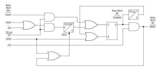
Note: The edge trigger timer associated with TCLOSDX starts on the rising edge of the input and outputs a pulse after CLOSDX ms.
