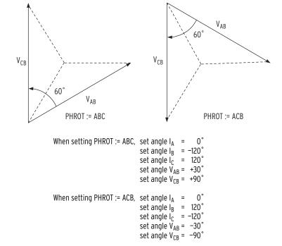
Figure 11.4 Three-Phase Open-Delta AC Connections
