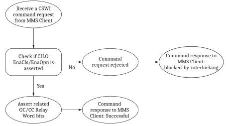
Figure G.6 CSWI Logical Node Direct Operate Command Request
