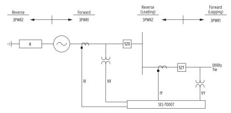
Figure 4.97 Power Elements Operation in the Real/Reactive Power Plane
