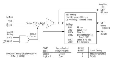
① From Figure 4.53 or Figure 4.54 ② From Figure 4.84 Figure 4.60 Neutral Time-Overcurrent Element 51NT
