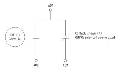
Figure 2.17 Output OUT103 Relay Output Contact Configuration
