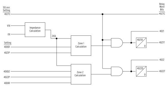
Figure 4.31 Loss-of-Field Logic Diagram
