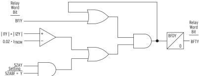
Figure 4.148 Breaker Failure Logic
