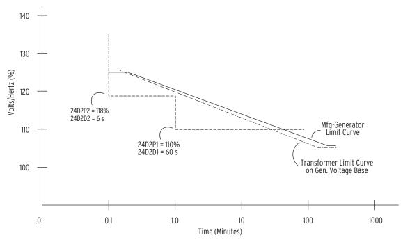
Dual-Level Volts/Hertz Time-Delay Characteristic 24CCS = DD
