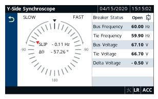
Figure 8.44 Y-Side Synchroscope
