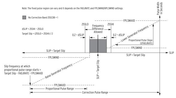
Figure 4.121 Frequency Correction Characteristics
