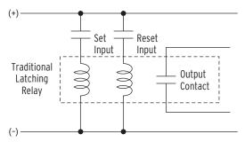
Figure 4.141 Schematic Diagram of a Traditional Latching Device
