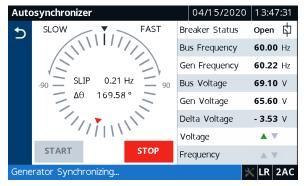
Figure 8.60 Generator Synchronizing
