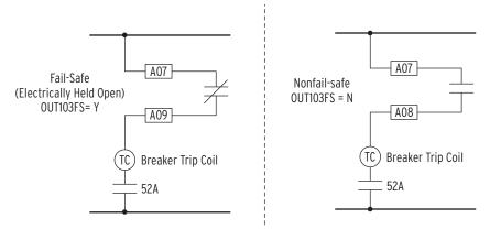
NOTE: Contacts shown with OUT103 relay coil de-energized
