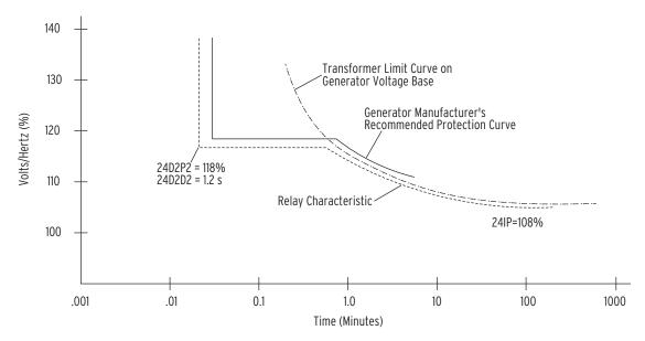
Figure 4.40 Composite Inverse/Definite-Time Overexcitation Characteristic, 24CCS = ID
