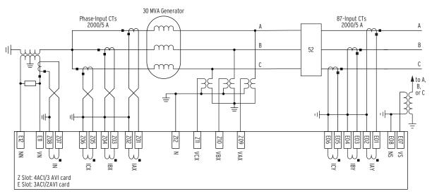
Figure 2.26 SEL-700G1+ Relay Typical AC Current and Four-Wire Wye Voltage Connection With MOT SEL-0700G11A2XBA76850231
