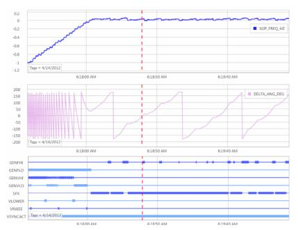
Figure 4.126 Graphical Display of Generator Autosynchronism Report
