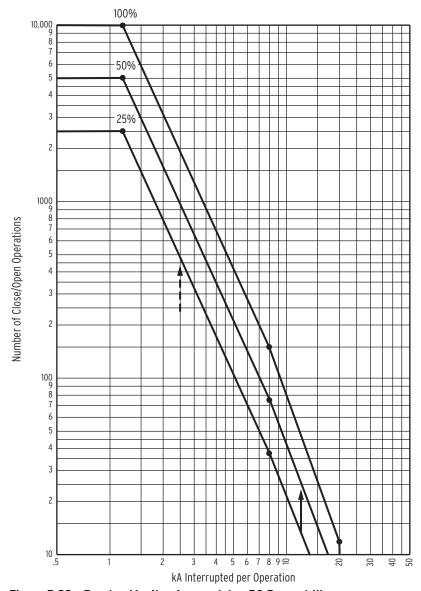
Figure 5.23 Breaker Monitor Accumulates 50 Percent Wear
