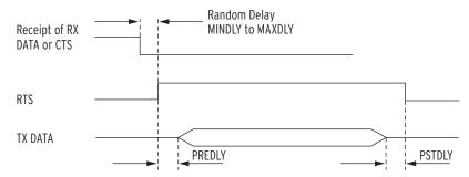
Figure D.2 Message Transmission Timing
