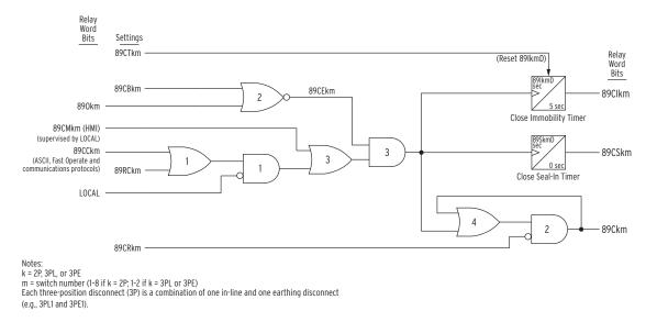
Figure 9.2 Disconnect Close Logic
