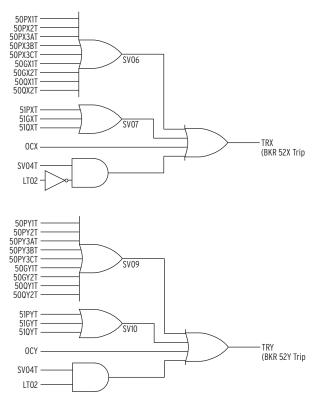
Figure 4.137 Typical Feeder Trip TR Logic (SEL-700GW)
