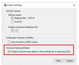
Figure G.1 Enable Functional Naming in Architect
