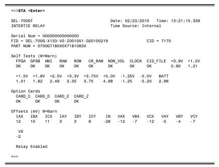
Figure 1.3 STA Command Response-No Communications Card or EIA-232/EIA-485 Communications Card
