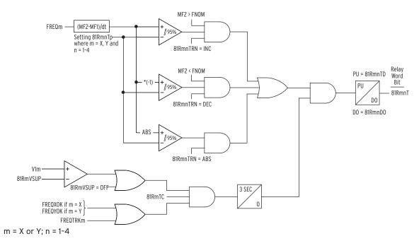
Figure 4.100 81R Frequency Rate-of-Change Scheme Logic
