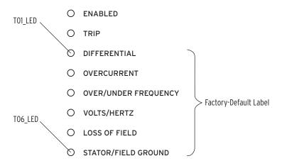
NOTE: There are three versions of factory-default front-panel LED configurations depending on the model (SEL-700G, SEL-700GT, or SEL-700GW).
