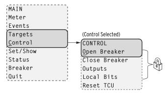
Figure 8.18 MAIN Menu and CONTROL Submenu
