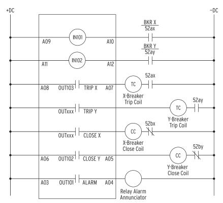
Figure 2.32 SEL-700GW Typical DC External Connections
