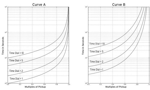
Figure 4.106 Inverse-Time Undervoltage Element Curves
