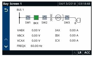
Figure 9.23 ANSI SEL-700G1 With GSU and Disconnects
