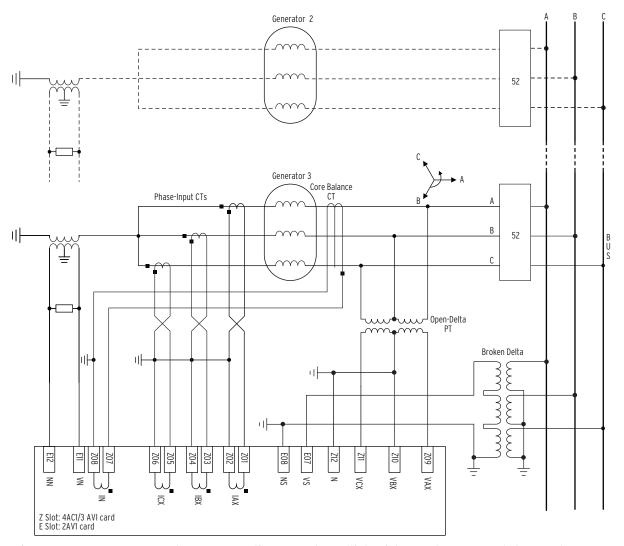
Figure 2.28 SEL-700G1+ Relay AC Connection Example, Multiple High-Impedance Grounded Generators Connected to a Common Bus, With 67N and Other Protection
