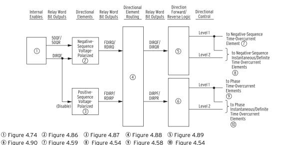
Figure 4.85 General Logic Flow of Directional Control for Negative-Sequence and Phase Overcurrent Elements (Apply Only to the Y Side of the SEL-700GT and SEL-700GT+ Relays)
