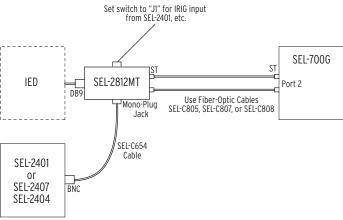
If you use Port 2 for the IRIG-B input, you cannot use a **B01-B02** input or Port 3 input. Set Global setting IRIG TIME SOURCE to TIME\_SRC := IRIG2.
