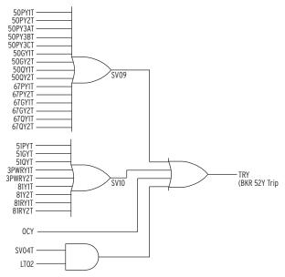
Figure 4.136 Typical Intertie Trip TR Logic (SEL-700GT)
