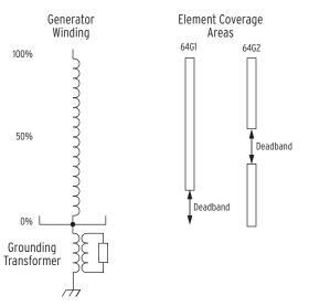
Figure 4.21 64G Element Operating Characteristic
