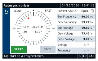
Figure 4.125 Auto Synchronizer Before Synchronization
