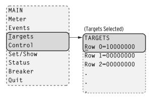
Figure 8.16 MAIN Menu and TARGETS Submenu
