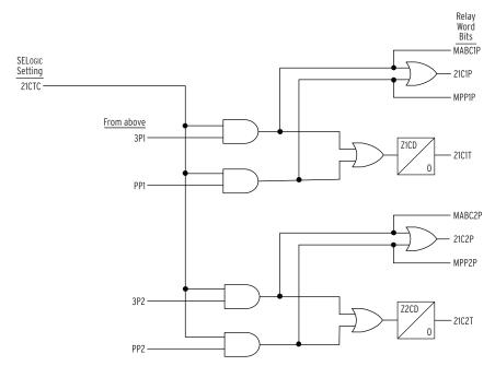
Figure 4.27 Compensator Distance Element Logic
