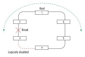
Figure 7.18 Physical Link Failure Between Devices
