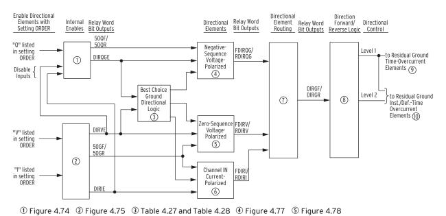
Figure 4.72 General Logic Flow of Directional Control for Residual Ground Overcurrent Elements
