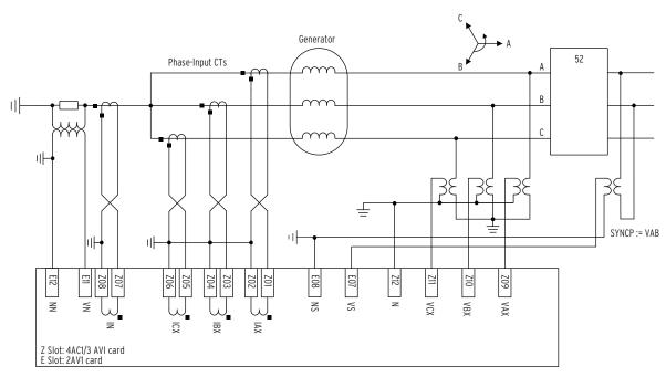
Figure 2.22 SEL-700G0+ Relay High-Impedance Grounded Generator With Synchronism Check and Without Current Differential Protection
