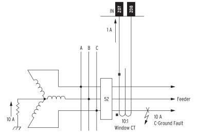
Figure 4.57 Ground Fault Protection Using Core-Balance CT
