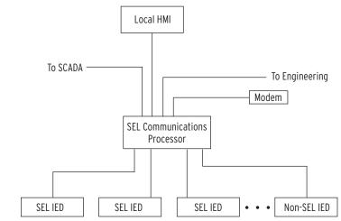
Figure C.1 SEL Communications Processor Star Integration Network
