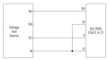
Figure 11.9 Delta Voltage Source Connections
