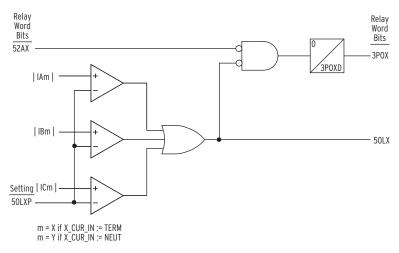
Figure 4.132 Pole Open Logic Diagram, Breaker 52X
