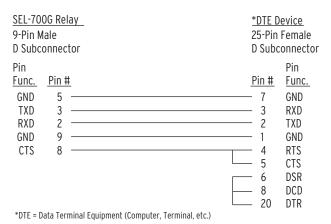
Figure 7.11 SEL-C227A Cable-SEL-700G to DTE Device
