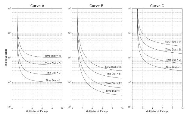
Figure 4.108 Inverse-Time Overvoltage Element Curves
