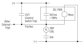
Figure 5.25 Input INxxx Connected to Trip Bus for Breaker Monitor Initiation
