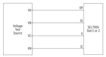
Figure 11.8 Wye Voltage Source Connections
