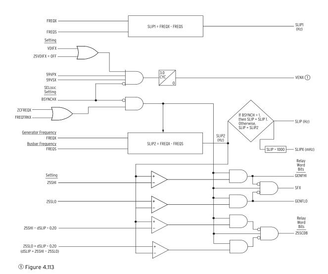
Figure 4.112 Synchronism-Check Function Slip Elements
