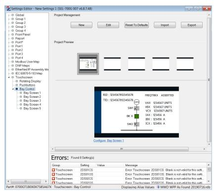
Figure 9.20 QuickSet Updated Single-Line Diagram and Corresponding Settings
