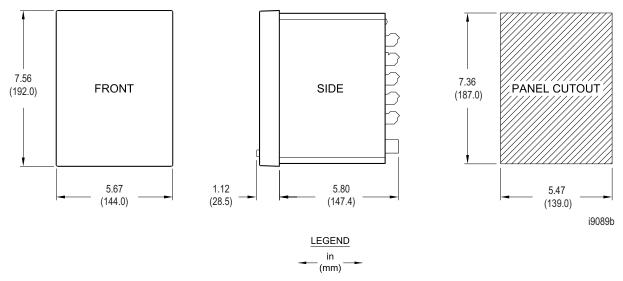
Figure 2.1 Relay Panel-Mount Dimensions
