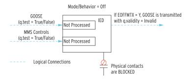
Figure G.14 Relay Operations in Off Mode
