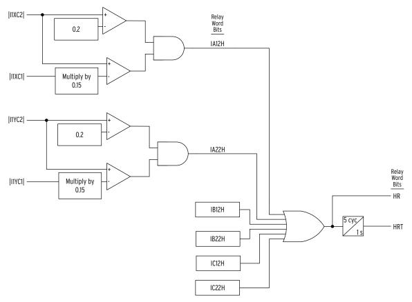
Figure 4.10 Second-Harmonic External Event Detector Logic
