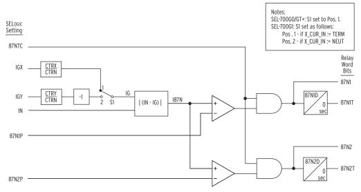
Figure 4.16 87N Element Logic Diagram
