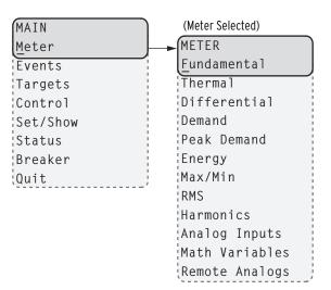
Figure 8.7 MAIN Menu and METER Submenu
