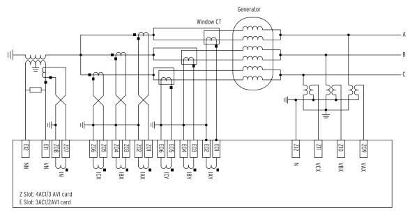
Figure 2.25 SEL-700G1+ Relay High-Impedance Grounded Generator With Split-Phase, **Self-Balancing Differential Protection**
