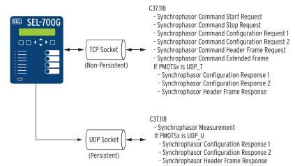
Figure K.5 UDP\_T and UDP\_U Connections
