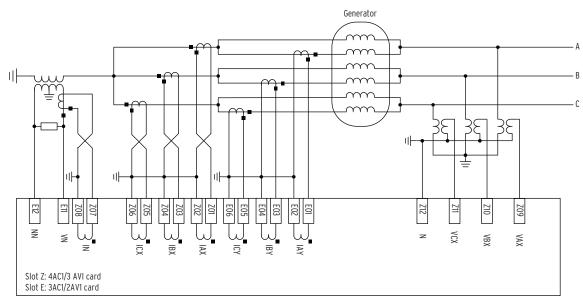
Figure 2.24 SEL-700G1+ Relay AC Connection Example-High-Impedance Grounded Generator With Split-**Phase Current Differential Protection**
