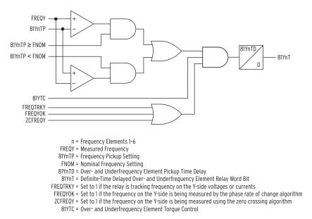
Figure 4.99 Y-Side Over- and Underfrequency Element Logic
