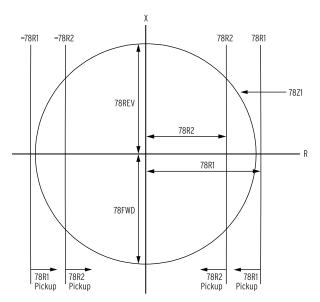
Figure 4.49 Double-Blinder Scheme Operating Characteristics
