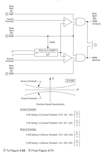
Figure 4.86 Negative-Sequence Voltage-Polarized Directional Element for Negative-Sequence and Phase Overcurrent Elements (Apply Only to the Y Side of the SEL-700GT and SEL-700GT+ Relays)
