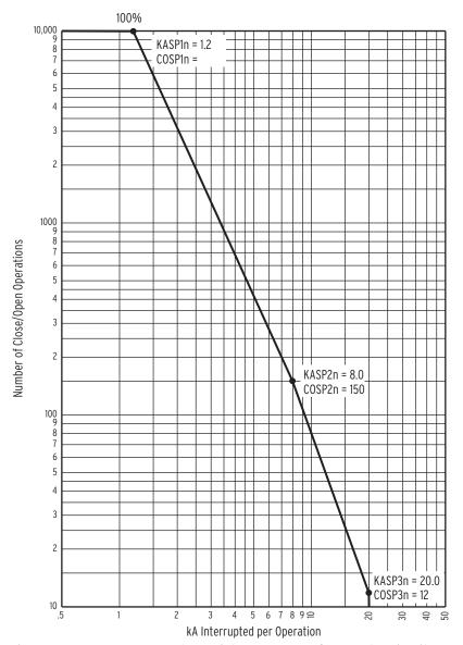
Figure 5.19 SEL-700G Breaker Maintenance Curve for a 25 kV Circuit Breaker
