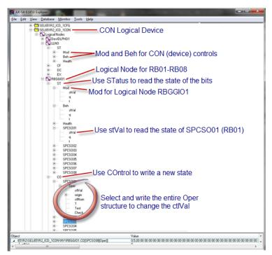
Figure G.7 MMS Client View of the CON Logical Device
