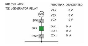
Figure 9.12 Bay Control Single-Line Diagram Schematic
