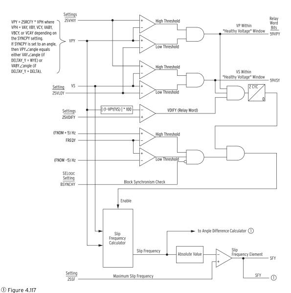
Figure 4.116 Synchronism-Check Voltage Window and Slip Frequency Elements
