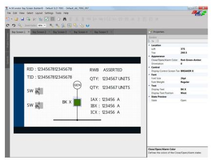
Figure 9.17 Selected Breaker Symbol Settings Displayed in the Properties Pane
