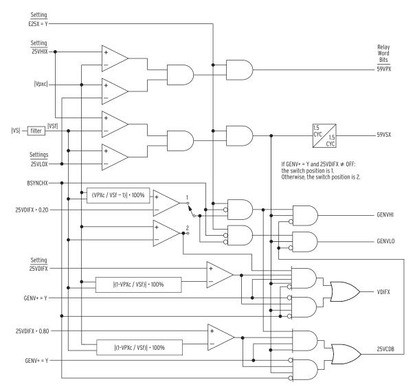
Vpxc = 25RCFX \* VP (where 25RCFX is the setting and VP is determined by the SYNCPX setting).
