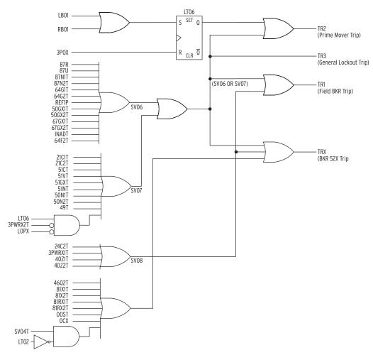
Figure 4.135 Typical Generator Trip TR Logic (SEL-700G0, SEL-700G1, SEL-700GT)
