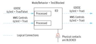
Figure G.13 Relay Operations in Test/Blocked Mode
