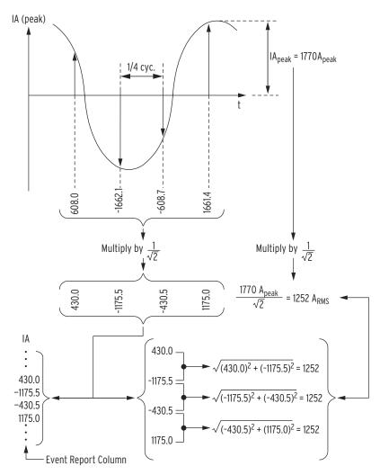
Figure 10.4 Derivation of Analog Event Report Current Values and RMS **Current Values From Sampled Current Waveform**
