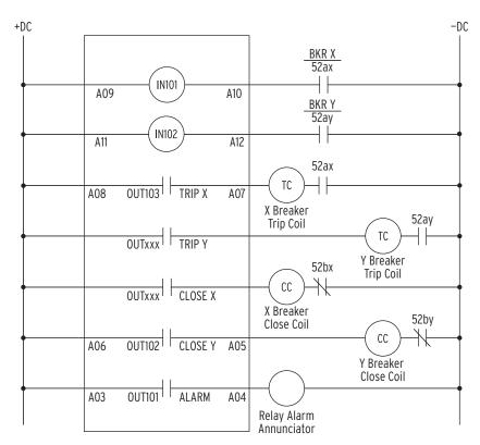
Figure 2.30 SEL-700GT+ Typical DC External Connections
