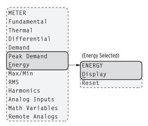
Figure 8.8 METER Menu and ENERGY Submenu
