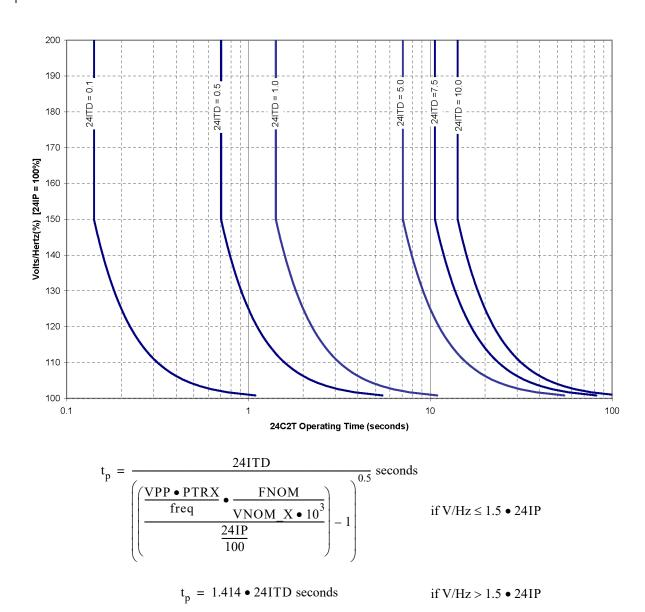
Figure 4.41 Volts/Hertz Inverse-Time Characteristic, 24IC = 0.5
