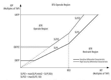
Figure 4.2 Percentage Restraint Differential Characteristic
