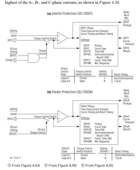
Figure 4.58 Maximum Phase Time-Overcurrent Elements
