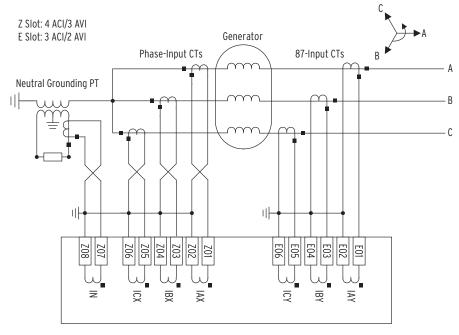
The current transformers and the SEL-700G chassis must be grounded in the relay cabinet.
