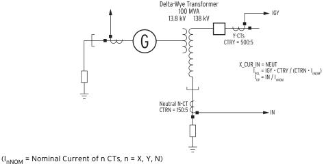
Figure 4.20 Effect of X\_CUR\_IN Setting on Polarizing Current
