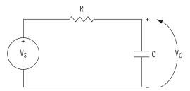
Figure 4.131 Voltage V<sub>S</sub> Applied to Series RC Circuit
