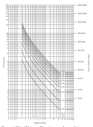
Figure 4.69 IEC Class C Curve (Extremely Inverse): C3
