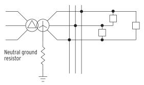
Figure 4.93 Hybrid Power System With Neutral-Ground Resistor
