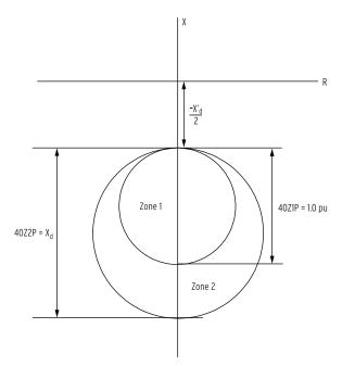
Figure 4.32 Loss-of-Field Element Operating Characteristic, Negative Zone 2 Offset
