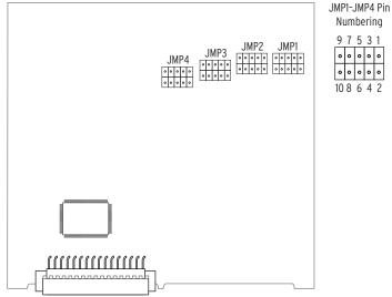
You need to insert three jumpers for a current analog output selection and two selection, insert a jumper between Pins 1 and 2, Pins 5 and 6, and Pins 9 and 10. For a voltage analog output selection, insert a jumper between Pins 3 and 4, and Pins 7 and 8. Figure 2.5 shows JMP4 selected as a current analog output. The current analog output selection is the default setting for JMP1 through JMP4. Figure 2.6 shows JMP1 selected as a voltage analog output.
