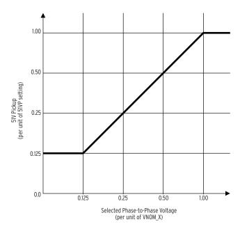
Figure 4.30 51V Element Voltage Restraint Characteristic
