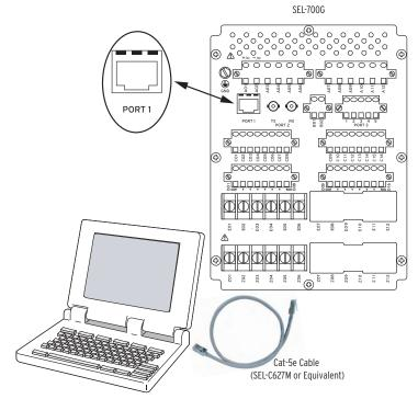
Figure 3.1 Direct Connection of SEL-700G to a Computer
