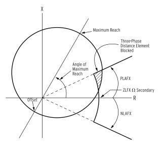
NOTE: The three-phase distance element operates for ABC faults. It is normal for it to operate for AB faults depending on the 50PPn pickup setting. The phase-to-phase element operates for AB, BC, and CA faults.
