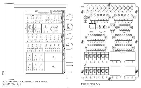
Figure 2.10 SEL-700GW With Copper Ethernet, 4 DI/4 DO, 4 AI/4 AO, 3 ACIE, 3 ACIZ (Relay MOT 0700GW1A1A6X77870310)
