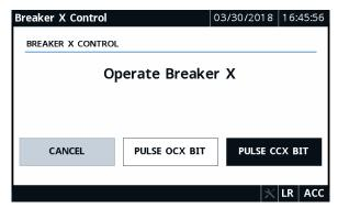
Figure 8.50 Breaker Control Selection
