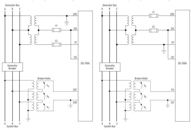
Figure 2.19 Voltage Connections
