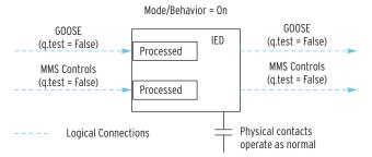
Figure G.10 Relay Operations in On Mode
