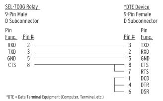
Figure 7.10 SEL-C234A Cable-SEL-700G to DTE Device
