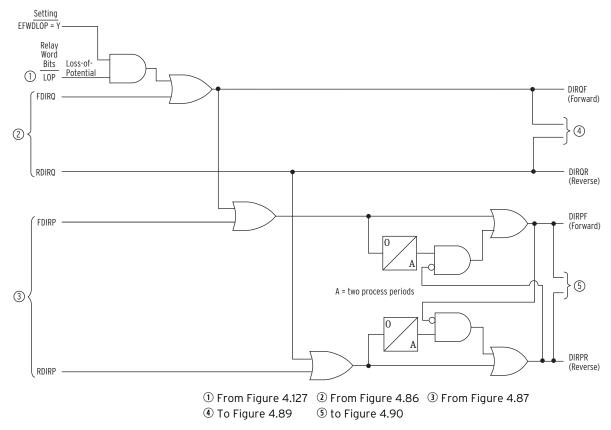
Figure 4.88 Routing of Directional Elements to Negative-Sequence and Phase Overcurrent Elements (Apply Only to the Y Side of the SEL-700GT and SEL-700GT+ Relays)
