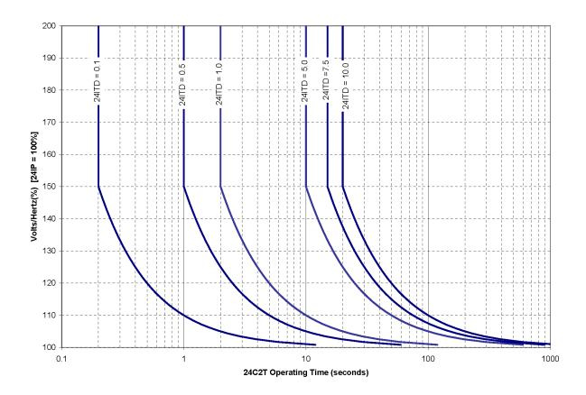
$$t_{p} = \frac{24ITD}{\left(\frac{\text{VPP} \bullet \text{PTRX}}{\text{freq}} \bullet \frac{\text{FNOM}}{\text{VNOM}\_X \bullet 10^{3}}\right) - 1} \text{seconds}$$
