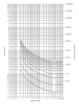
Figure 4.70 IEC Long-Time Inverse Curve: C4
