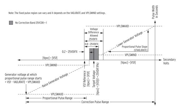
Figure 4.124 Voltage Connection Characteristics When GENV+ = Y
