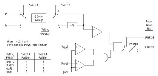
Figure 4.96 Three-Phase Power Elements Logic
