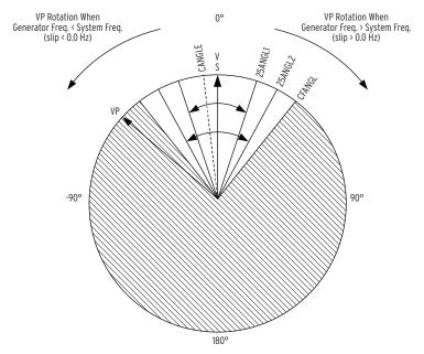
Figure 4.115 Synchronism-Check Function Angle Characteristics
