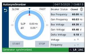
Figure 8.62 Generator Synchronized
