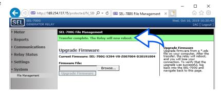
**NOTE:** After the relay reboots, if the **ENABLED** LED is not illuminated or if the front panel displays STATUS FAIL Non\_Vol Failure on the two-line display model, or a settings mismatch notification screen on the touchscreen model, then open a terminal emulator using the serial port and use the following procedure to restore the factory-default settings. Refer to Upgrade the Firmware Using a Terminal Emulator for terminal emulator setup and connections.
