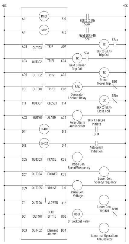
Figure 2.27 SEL-700G1+ Typical DC External Connections
