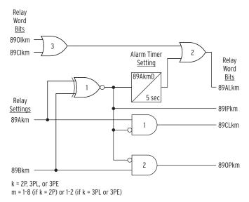
Figure 9.1 Dual-Point Disconnect Status Logic
