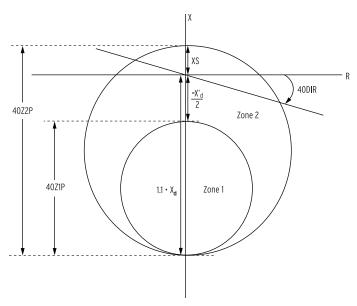
Figure 4.33 Loss-of-Field Element Operating Characteristic, Positive Zone 2 Offset
