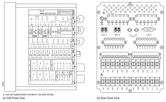
Figure 2.8 SEL-700G1+ With Dual-Fiber Ethernet, Fast Hybrid 4 DI/4 DO, 10 RTDs, 3 ACI/2 AVI, 4 ACI/3 AVI (Relay MOT 0700G11ACA9X76850830)
