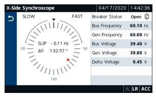
Figure 8.43 X-Side Synchroscope
