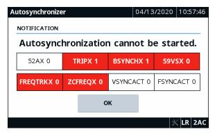
Figure 8.59 Auto Synchronizer Cannot Be Started
