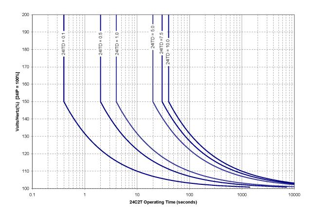
$$t_{p} = \frac{24ITD}{\left(\frac{\text{VPP} \bullet \text{PTRX}}{\text{freq}} \bullet \frac{\text{FNOM}}{\text{VNOM}_{\perp} X \bullet 10^{3}} - 1\right)^{2.0}} \text{ seconds} \quad \text{if V/Hz} \le 1.5 \bullet 24IP$$
