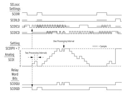
Figure 4.147 Example of the Effects of the Input Precedence
