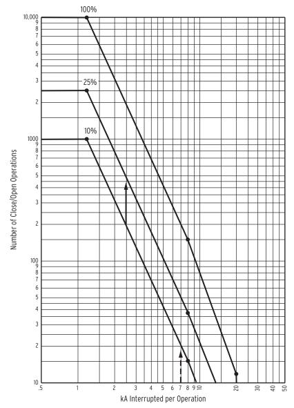
Figure 5.22 Breaker Monitor Accumulates 25 Percent Wear
