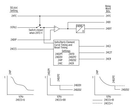
Figure 4.38 Volts/Hertz Element Logic
