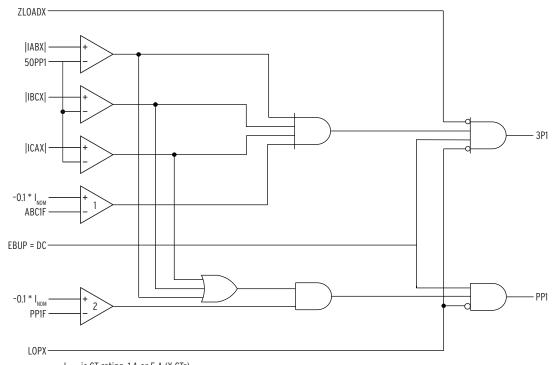
$I_{\text{NOM}}$  is CT rating, 1 A or 5 A (X-CTs). ABC1F and PP1F are values calculated by compensator distance element. Zone 2 logic is similar to Zone 1.
