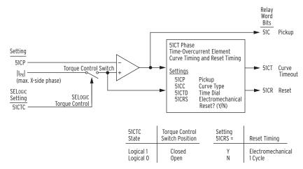
Figure 4.28 Voltage-Controlled Phase Time-Overcurrent Element 51CT
