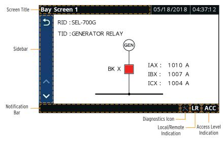
Figure 8.29 Touchscreen Display Components and Indicators
