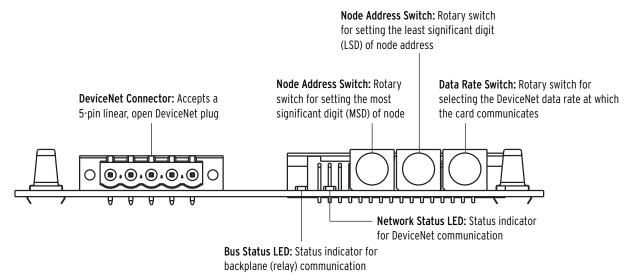
Figure I.1 DeviceNet Card Component Overview
