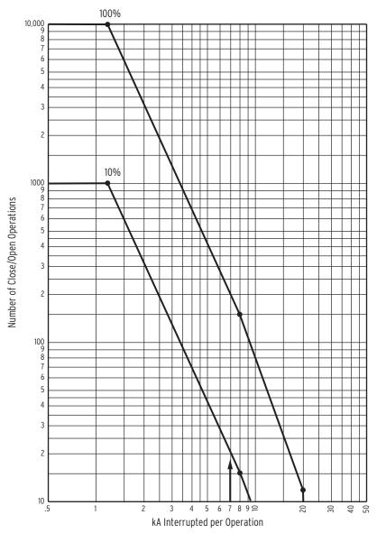
Figure 5.21 Breaker Monitor Accumulates 10 Percent Wear
