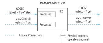
Figure G.12 Relay Operations in Test Mode
