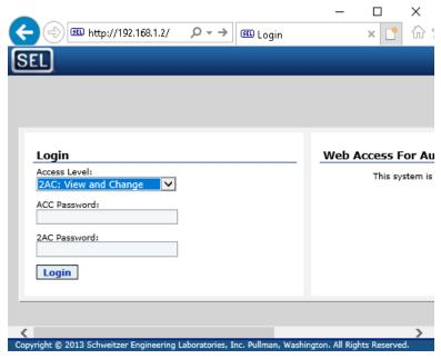
Figure 3.3 Selecting Access Level 2 From Web Server Login
