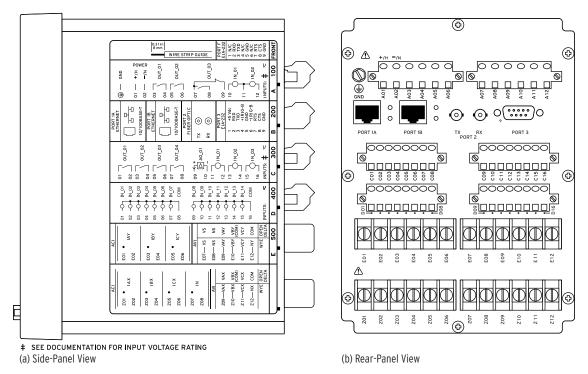
Figure 2.11 SEL-700GT+ With Dual Copper Ethernet, 3 DI/4 DO/1 AO, 14 DI, 3 ACI/4 AVI on Slot E, 4 ACI/3 AVI on Slot Z (Relay MOT 0700GT1ABA4A7585A670)
