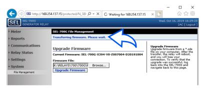
After the relay finishes the firmware transfer, an acknowledgment message appears and the relay reboots.
