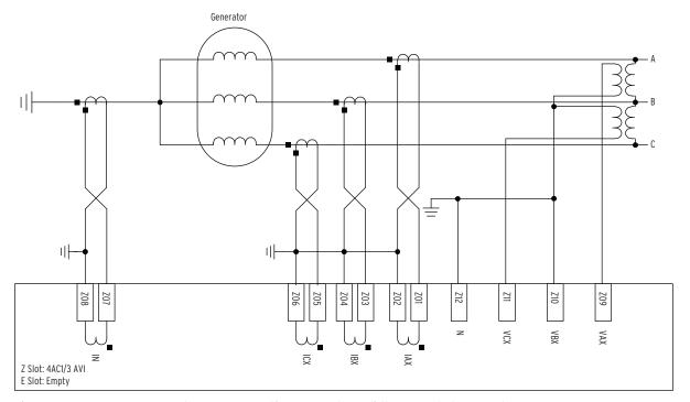
Figure 2.21 SEL-700G0 Relay AC Connection Example-Solidly Grounded Generator With Ground Differential Protection (87N)
