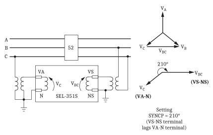
Figure 3.27 Example Single-Phase VA-N With Phase-to-Phase VS-NS Synchronism-Check Voltage
