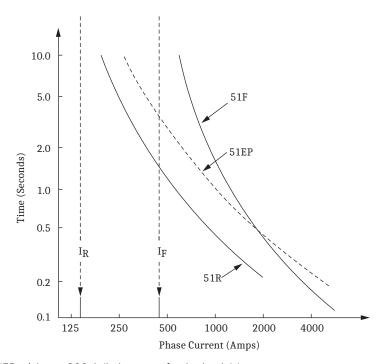
51EP: pickup = 300 A (below max. feeder load,  $I_F$ )
