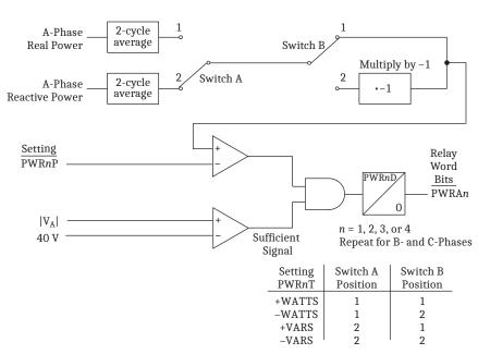
Figure 3.45 Single-Phase Power Elements Logic (+VARS Example Shown)
