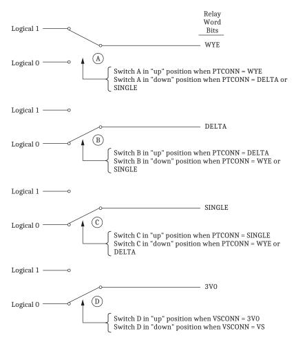
Figure 9.21 Operation of WYE, DELTA, SINGLE, and 3VO Relay Word Bits
