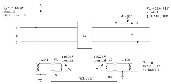
Figure 3.30 Example System With Synchronism-Check Voltage Connected Phase-To-Phase
