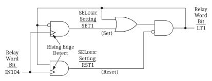
Figure 7.14 Latch Control Switch Controlled by a Single Input to Enable/Disable Reclosing
