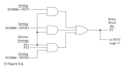
Figure 5.5 Permissive Input Logic Routing to POTT Logic
