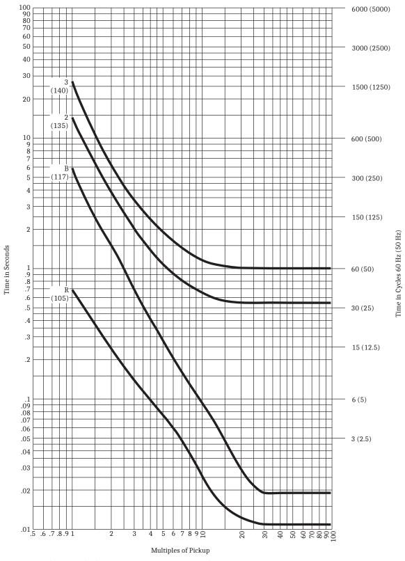
Figure 9.12 Recloser Control Response Curves B, R, 2, and 3
