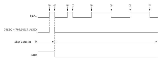
① Fault occurs beyond line recloser. ② Fault cleared by line recloser fast curve. ③ Line recloser recloses into fault. ④ Fault cleared by line recloser slow curve.
