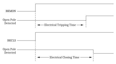
Figure 8.9 Electrical Operating Time
