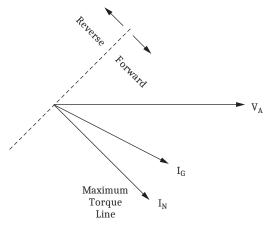
Figure 4.30 Traditional Channel IN Current-Polarized Directional Element
