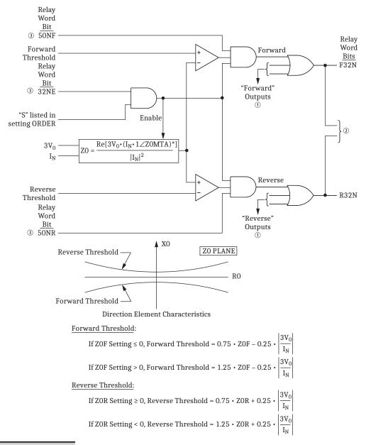
**NOTE:** Residual ground current  $I_G$  is used in place of neutral current  $I_N$  under certain conditions. See Switch Between  $I_N$  and  $I_G$  for Low-Impedance Grounded and Ungrounded/High-Impedance Grounded Systems on page 4.20.
