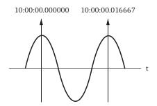
Figure N.1 High-Accuracy Clock Controls Reference Signal (60 Hz System)
