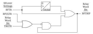
Figure 5.19 Breaker Failure Trip Logic
