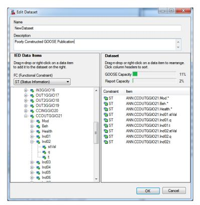
Figure P.3 Example of a Poorly Constructed GOOSE Dataset
