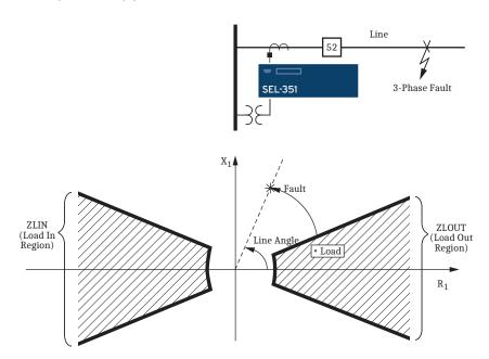
Figure 4.7 Migration of Apparent Positive-Sequence Impedance for a Fault Condition
