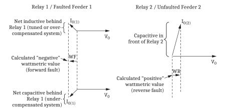
Figure 4.41 Wattmetric Element Operation for Ground Fault on Feeder 1
