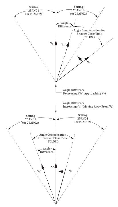
Figure 3.33 Angle Difference Between  $V_P$  and  $V_S$  Compensated by Breaker Close Time ( $f_P < f_S$  and  $V_P$  Shown as Reference in This Example)
