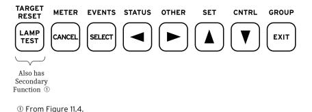
Figure 11.1 SEL-351S Front-Panel Pushbuttons-Overview
