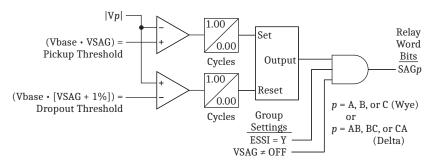
Figure 3.41 Voltage Sag Elements
