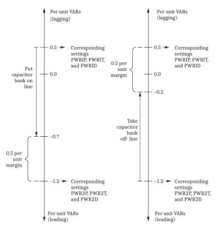
Figure 3.49 Per Unit Setting Limits for Switching 9600 kVAR Capacitor Bank On- and Off-Line
