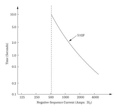
Figure G.5 Negative-Sequence Overcurrent Element Derived From Equivalent Phase Overcurrent Element, 51EP
