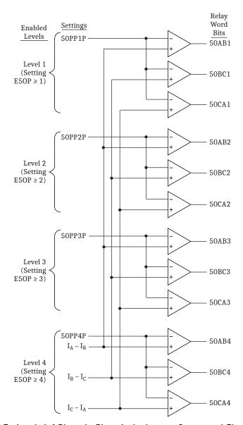
Figure 3.7 Levels 1-4 Phase-to-Phase Instantaneous Overcurrent Elements
