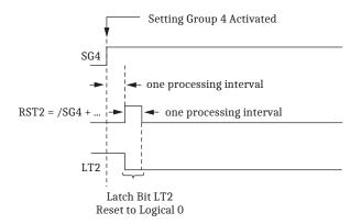
Figure 7.16 Time Line for Reset of Latch Bit LT2 After Active Setting Group Change
