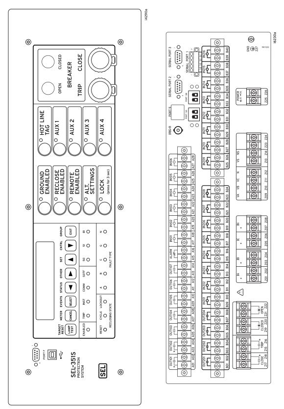
Figure 2.4 SEL-351S Front- and Rear-Panel Drawings; Horizontal Panel-Mount With Optional Front-Panel USB Port and SafeLock Trip/Close Pushbuttons, Optional Extra I/O Board With 4 Standard Outputs and 16 Inputs, Optional Dual Fiber-Optic Ethernet, and EIA-485 Port
