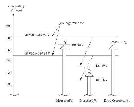
Figure 3.31 25RCF Settings Example Showing V<sub>A</sub> Adjustment
