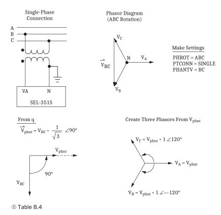
Figure 8.13 Example Phasor Diagram of Phantom Voltage Adjustment
