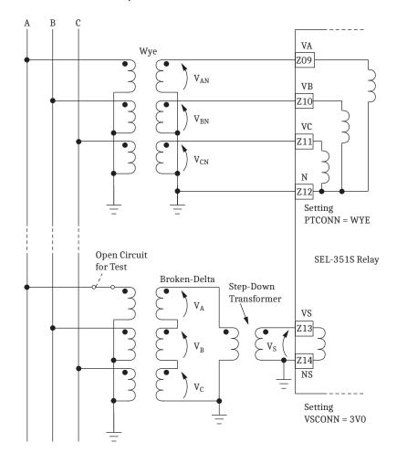
Figure 2.8 Broken-Delta Secondary Connection to Voltage Input VS, Wye-Connected PTs
