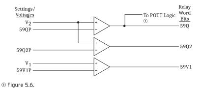
Figure 3.25 Sequence Voltage Elements (Delta-Connected PTs)
