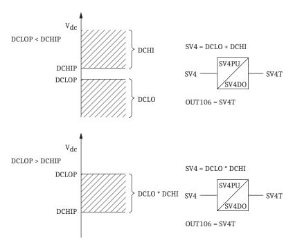
Figure 8.12 Create DC Voltage Elements With SELogic Control Equations
