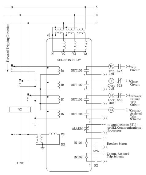
Voltage Channel **VS** does not need to be connected. Here, it is shown connected for use in voltage and synchronism-check elements and voltage metering. See Synchronism Check VS Connection (Global Setting VSCONN = VS) on page 2.14 and Broken-Delta VS Connection (Global Setting VSCONN = 3VO) on page 2.14.
