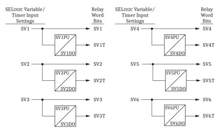
Figure 7.24 SELOGIC Control Equation Variables/Timers SV1/SV1T-SV6/SV6T
