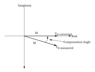
Figure N.3 Correction of Measured Phase Angle
