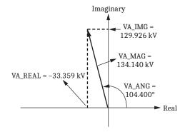
Figure N.4 Example Calculation of Real and Imaginary Components of Synchrophasor
