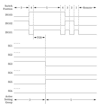
Figure 7.23 Active Setting Group Switching (With Rotating Selector Switch)
