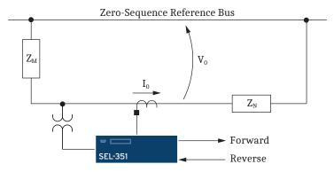
Figure 4.32 Zero-Sequence Impedance Network and Relay Polarity
