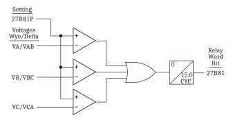
Figure 3.34 Undervoltage Block for Frequency Elements (Group Setting VNOM  $\neq$  OFF)
