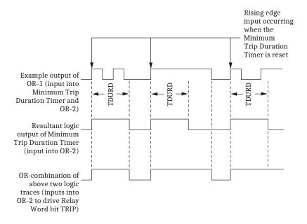
Figure 5.2 Minimum Trip Duration Timer Operation (See Bottom of Figure 5.1)
