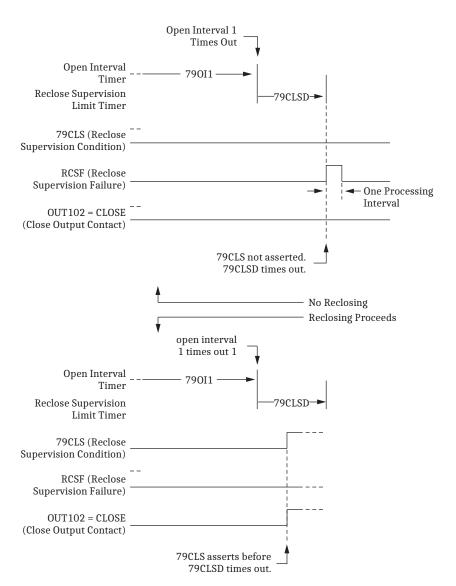
Figure 6.7 Reclose Supervision Limit Timer Operation (Refer to Bottom of *Figure 6.6*)
