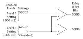
Figure 3.11 Levels 5-6 Residual Ground Instantaneous Overcurrent Elements
