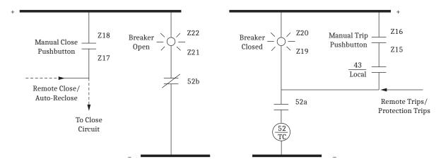
Figure 2.28 SEL-351S Example Wiring Diagram Using the SafeLock Trip/Close Pushbuttons
