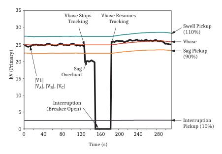
Figure 3.44 Vbase Tracking Example (Three-Phase Disturbance, Wye-Connected)
