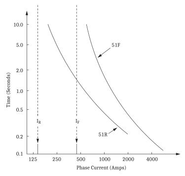
51F: pickup = 600 A (above max. feeder load,  $\rm I_F$ ); 51R: pickup = 200 A (above max. line recloser load,  $\rm I_R$ )
