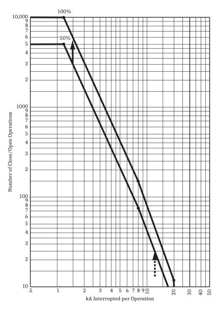
Figure 8.7 Breaker Monitor Accumulates 100 Percent Wear
