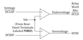
Figure 8.11 DC Under- and Overvoltage Elements
