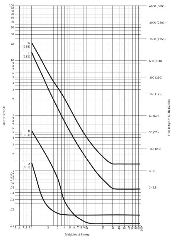
Figure 9.11 Recloser Control Response Curves A, C, N, and W
