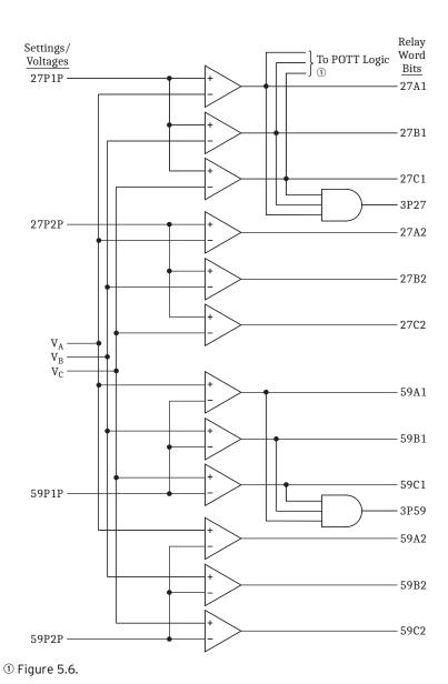
Figure 3.22 Single-Phase and Three-Phase Voltage Elements (Wye-Connected or Single-Phase-Connected PTs)
