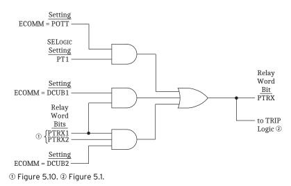
Figure 5.7 Permissive Input Logic Routing to Trip Logic
