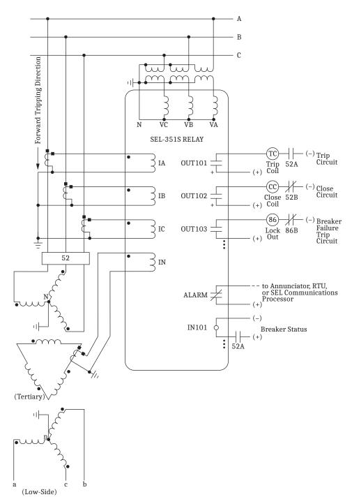
The voltage inputs do not need to be connected. Voltage is needed for voltage elements, synchronism-check elements, frequency elements, voltage-polarized directional elements, fault location, metering (i.e., voltage, MW, MVAR), frequency tracking, and frequency estimation.
