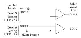
Figure 3.2 Levels 5-6 Phase Instantaneous Overcurrent Elements
