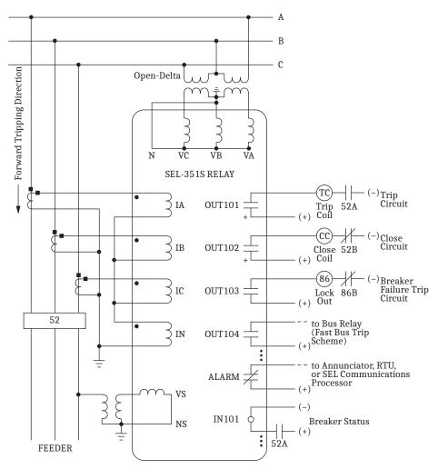
The voltage inputs can accept open-delta PT (three-wire) connection (as shown) when Global setting PTCONN = DELTA. **VB** (terminal Z10) must be externally tied to **N** (terminal Z12), as shown.
