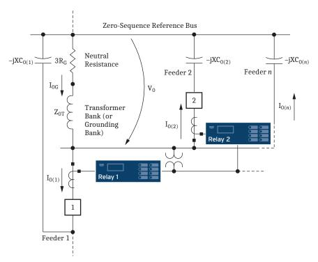
Figure 4.35 Zero-Sequence Impedance Network for Low-Impedance Grounded Distribution System With a Ground Fault on Feeder 1
