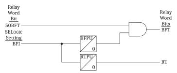
Figure 5.18 Breaker Failure Logic
