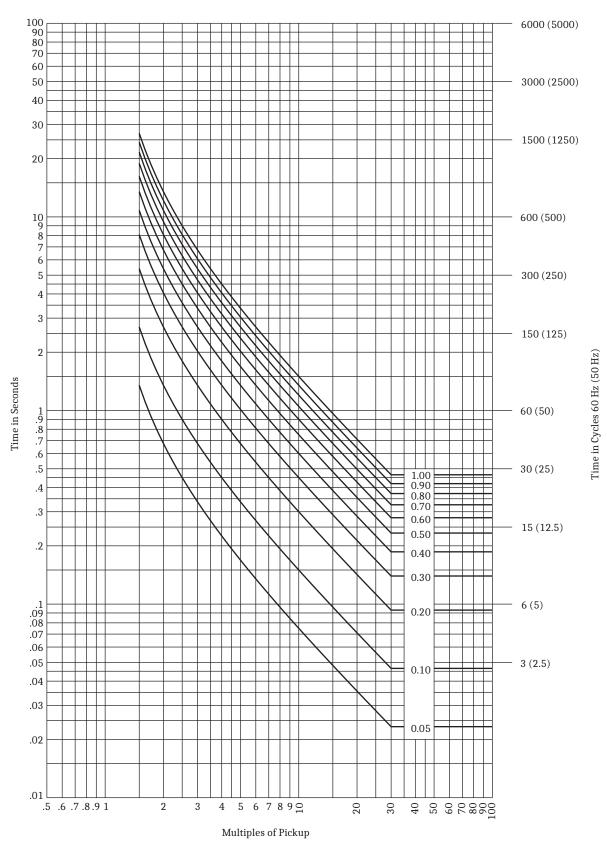
Figure 9.7 IEC Very Inverse (Class B) Curve (C2)
