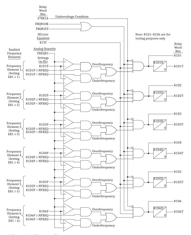
Figure 3.39 Levels 1-6 Frequency Elements
