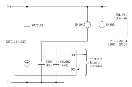
Figure 5.12 SEL-351S Connections to Communications Equipment for a Two-Terminal Line DCUB Scheme (Setting ECOMM = DCUB1)
