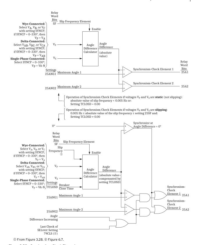
Figure 3.29 Synchronism-Check Elements
