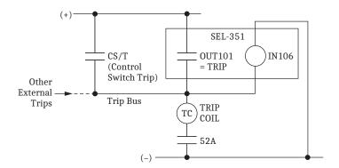
Figure 8.10 Input IN106 Connected to Trip Bus for Breaker Monitor Initiation
