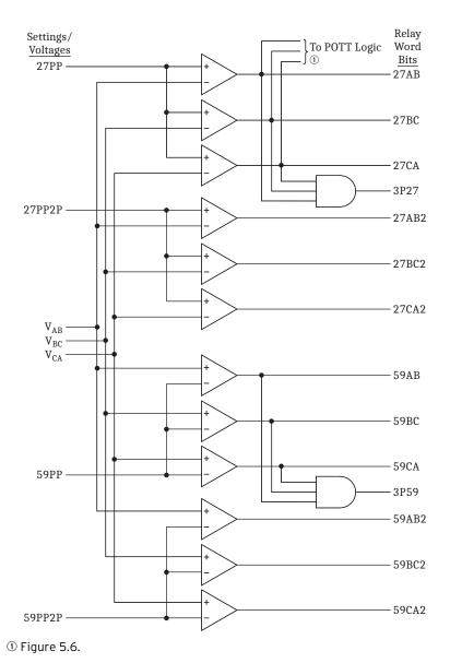
Figure 3.24 Phase-to-Phase Voltage Elements (Delta-Connected PTs)
