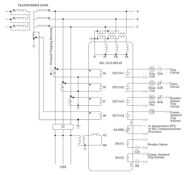
Voltage Channel VS does not need to be connected. Here, it is shown connected for use in voltage and synchronismcheck elements and voltage metering. See Synchronism Check VS Connection (Global Setting VSCONN = VS) on page 2.14 and Broken-Delta VS Connection (Global Setting VSCONN = 3VO) on page 2.14.
