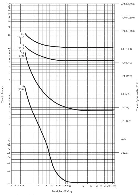
Figure 9.19 Recloser Control Response Curves 4, 9, 11, and 14
