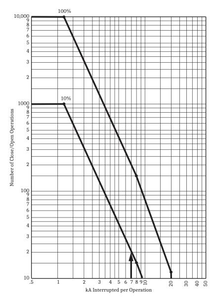
Figure 8.4 Breaker Monitor Accumulates 10 Percent Wear
