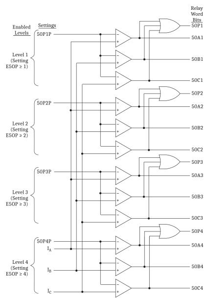
Figure 3.1 Levels 1-4 Phase Instantaneous Overcurrent Elements
