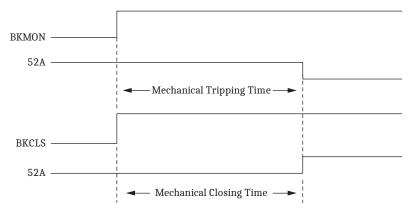
Figure 8.8 Mechanical Operating Time
