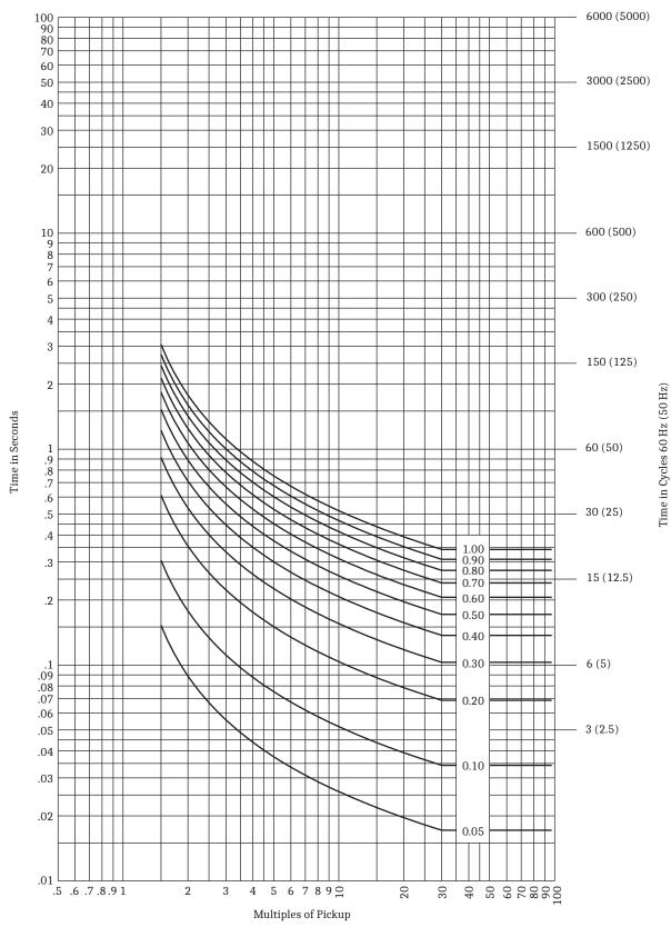
Figure 9.10 IEC Short-Time Inverse Curve (C5)
