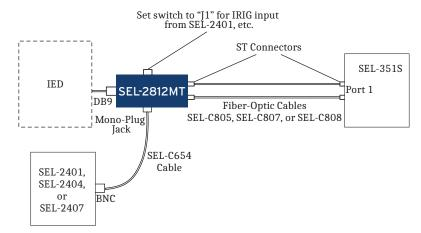
Figure 2.13 IRIG-BInput Via Fiber-Optic Port1(SEL-2401/SEL-2404/SEL-2407 Time Source)
