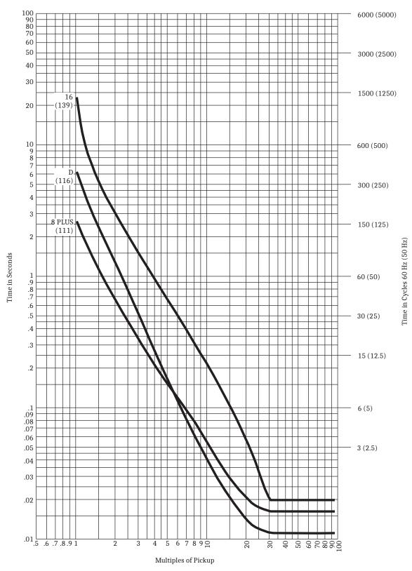
Figure 9.13 Recloser Control Response Curves D, 8 PLUS, and 16
