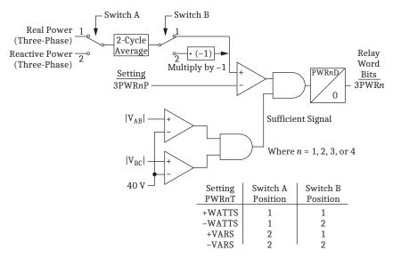
Figure 3.46 Three-Phase Power Elements Logic
