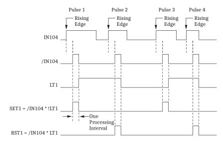
Figure 7.15 Latch Control Switch Operation Time Line
