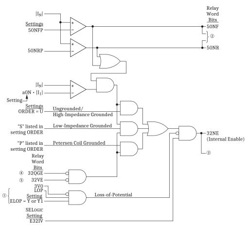
① From Figure 4.1. ② To Figure 4.17 and Figure 4.19. ③ To Figure 4.8, Figure 4.9, Figure 4.17, Figure 4.18, Figure 4.19, Table 4.4, and Table 4.5. ④ From Figure 4.11. ⑤ From Figure 4.12.
