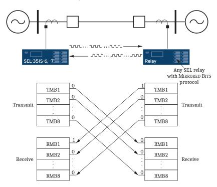
Figure H.1 Relay-to-Relay Logic Communication
