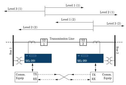
Figure 5.4 Communications-Assisted Tripping Scheme
