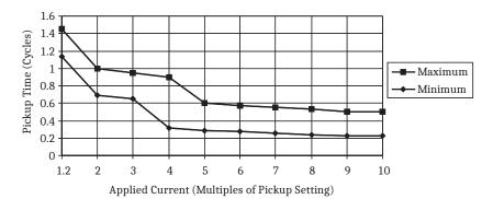
Figure 3.5 SEL-351S Nondirectional Instantaneous Overcurrent Element Pickup Time Curve
