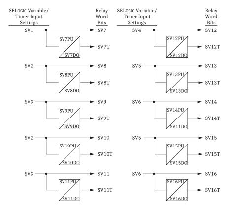
Figure 7.25 SELogicControlEquationVariables/TimersSV7/SV7T-SV16/SV16T
