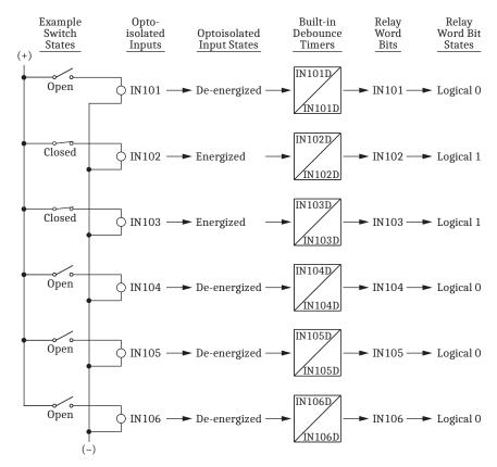
Figure 7.1 Example Operation of Optoisolated Inputs IN101-IN106 (All Models)
