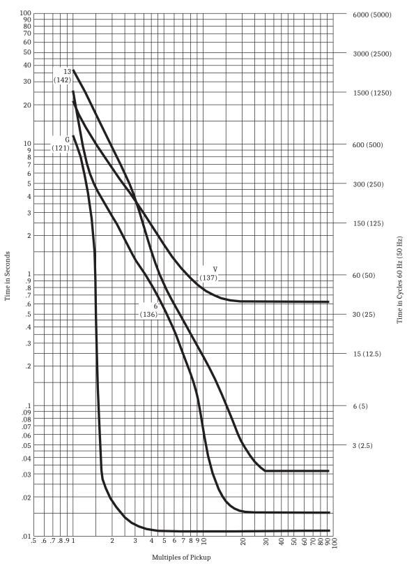
Figure 9.15 Recloser Control Response Curves G, V, 6, and 13
