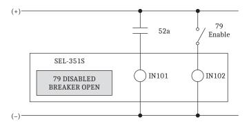
Figure 7.31 Rotating Display Replaces Traditional Panel Light Installations
