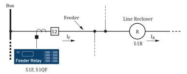
$I_F$  = Maximum load current through feeder relay = 450 A;  $I_R$  = Maximum load current through line recloser = 150 A; 51F = Feeder relay phase time-overcurrent element; 51QF = Feeder relay negative-sequence time-overcurrent element; 51R = Line recloser phase time-overcurrent element (phase "slow curve")
