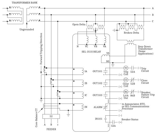
A core-balance current transformer is often referred to as a zero-sequence, ground fault, or window current transformer.
