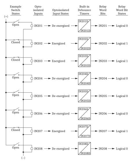
Figure 7.2 Example Operation of Optoisolated Inputs IN201-IN208
