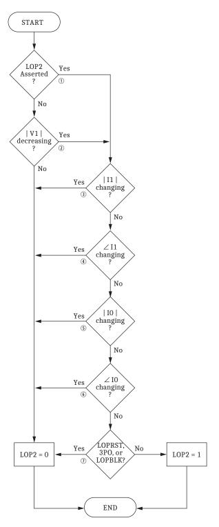
Figure 4.3 LOP2 Logic Processing Overview (Relay Word Bit LOP2)
