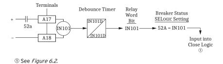
Figure 6.5 Breaker Status Determination
