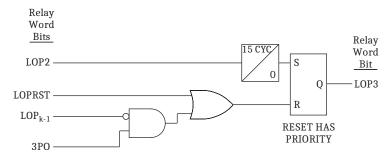
Figure 4.4 LOP Latch Logic (Relay Word Bit LOP3)
