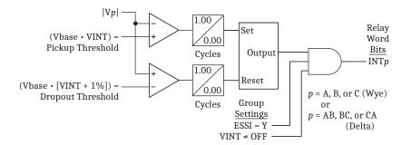
Figure 3.43 Voltage Interruption Elements
