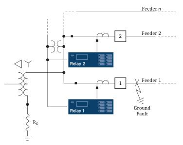
Figure 4.34 Low-Impedance Grounded Distribution System With a Ground Fault on Feeder 1
