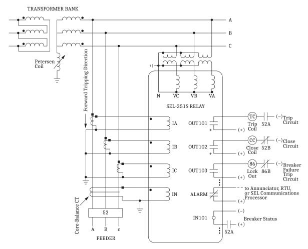
A core-balance current transformer is often referred to as a zero-sequence, ground fault, or window current transformer. Directional control for a Petersen Coil grounded system is selected with setting ORDER containing P (see Table 4.4-Table 4.6). Nondirectional sensitive earth fault (SEF) protection is also available.
