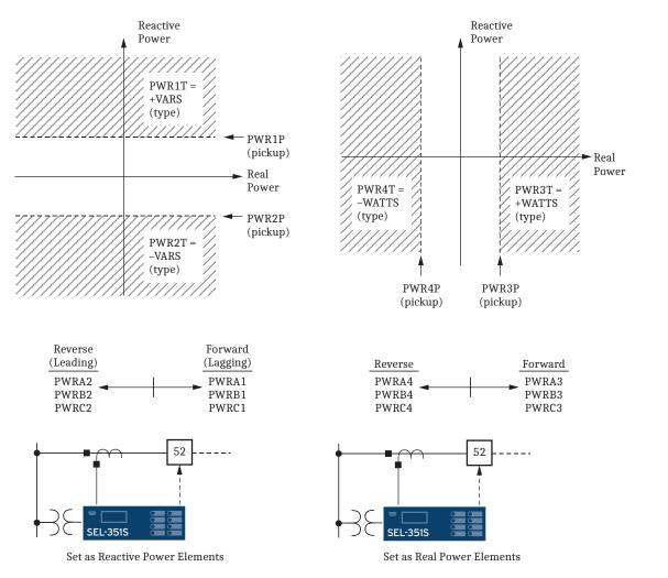
Figure 3.47 Power Elements Operation in the Real/Reactive Power Plane
