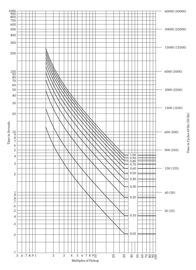
Figure 9.9 IEC Long-Time Inverse Curve (C4)
