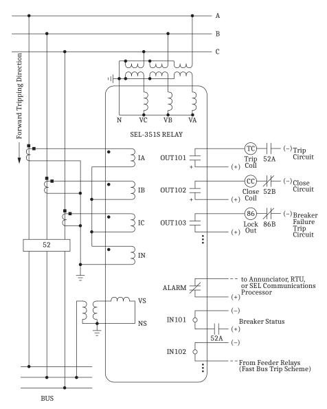
The fast bus trip scheme is often referred to as a reverse-interlocking or zone-interlocking scheme.
