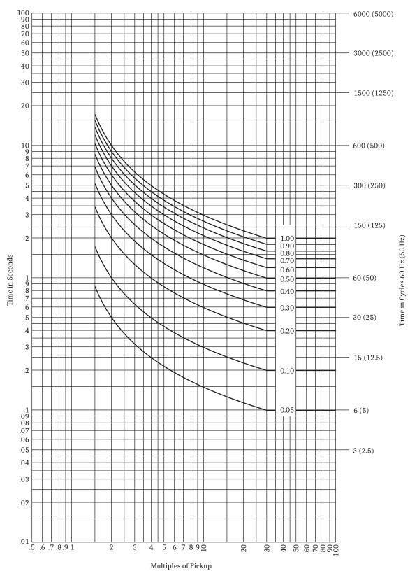
Figure 9.6 IEC Standard Inverse (Class A) Curve (C1)
