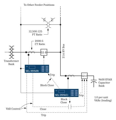
Figure 3.48 SEL-351S(B) Provides VAR Control for 9600 kVAR Capacitor Bank
