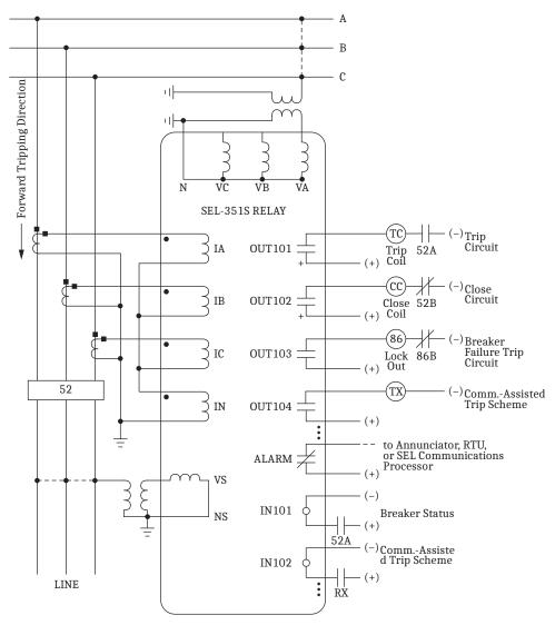
Voltage must be applied between relay terminals VA and N (209 and Z12, respectively) to deassert the undervoltage block of the frequency elements (setting 27B81P). Make Global setting PTCONN = SINGLE.
