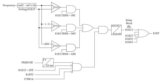
Logic shown for 81R1T. Logic for 81R2T-81R4T is similar.
