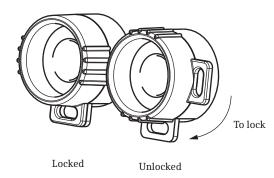
Figure 2.6 SafeLock Trip and Close Pushbuttons
