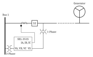
Figure 6.12 Reclose Blocking for Islanded Generator
