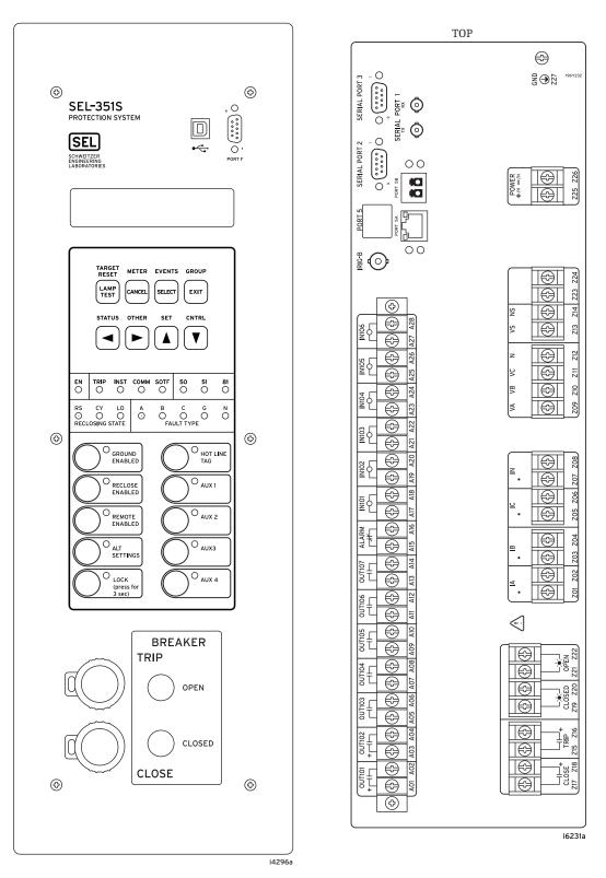
Figure 2.5 SEL-351S Front- and Rear-Panel Drawings; Vertical Panel-Mount With Optional Front-Panel USB Port and SafeLock Trip/Close Pushbuttons and Optional Dual Copper/Fiber-Optic Ethernet With Fiber-Optic Serial Port
