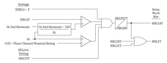
Figure 3.21 Second Harmonic Blocking Logic
