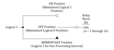
Figure 7.4 Local Control Switches Drive Local Bits LB1-LB16
