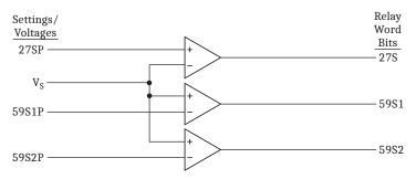
Figure 3.26 Channel VS Voltage Elements (Wye- or Delta-Connected PTs)
