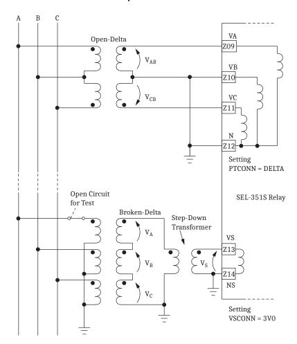
Figure 2.10 Broken-Delta Secondary Connection to Voltage Input VS, Open-Delta Connected PTs
