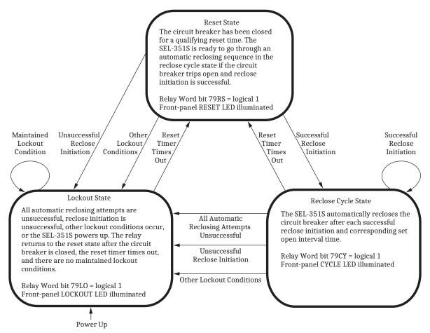
Figure 6.9 Reclosing Relay States and General Operation
