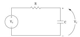
Figure 8.15 Voltage V<sub>S</sub> Applied to Series RC Circuit
