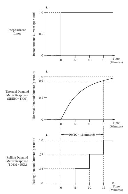
Figure 8.14 Response of Thermal and Rolling Demand Meters to a Step Input (Setting DMTC = 15 Minutes)
