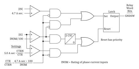
Figure 4.10 Logic for Relay Word Bit GNDSW
