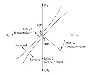
Figure 4.39 ZOMTA Setting Provides Forward/Reverse Ground Fault Discrimination in a Low-Impedance Grounded Distribution System
