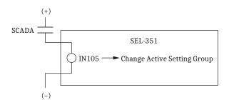
Figure 7.19 SCADA Contact Pulses Input IN105 to Switch Active Setting Group Between Setting Groups 1 and 4
