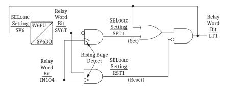
Figure 7.17 Latch Control Switch (With Time Delay Feedback) Controlled by a Single Input to Enable/Disable Reclosing
