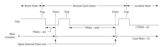
Figure 6.10 Example Reclosing Sequence From Reset to Lockout
