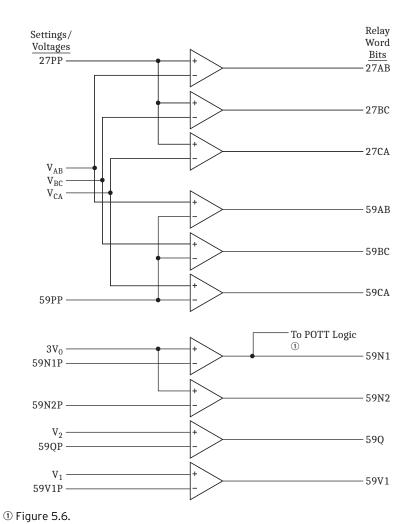
Figure 3.23 Phase-to-Phase and Sequence Voltage Elements (Wye-Connected PTs)
