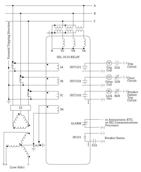
The voltage inputs do not need to be connected. Voltage is needed for voltage elements, synchronism-check elements, frequency elements, voltage-polarized directional elements, fault location, metering (i.e., voltage, MW, MVAR), frequency tracking, and frequency estimation.
