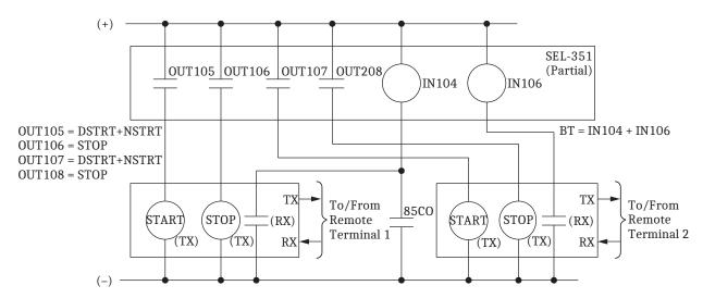
Figure 5.16 SEL-351S Connections to Communications Equipment for a Three-Terminal Line DCB Scheme
