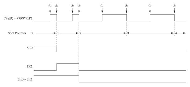
1 Fault occurs beyond line recloser. 2 Fault cleared by line recloser fast curve. 3 Line recloser recloses into fault. 4 Fault cleared by line recloser slow curve.
