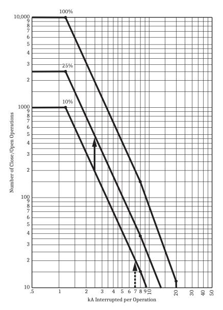
Figure 8.5 Breaker Monitor Accumulates 25 Percent Wear
