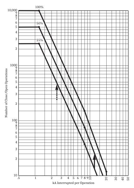
Figure 8.6 Breaker Monitor Accumulates 50 Percent Wear
