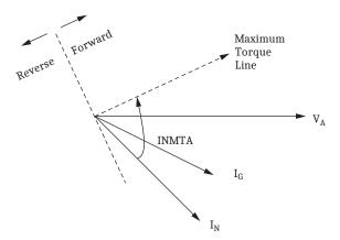
Figure 4.31 Current-Polarized Directional Element Characteristic When INMTA  $\neq$  0.00
