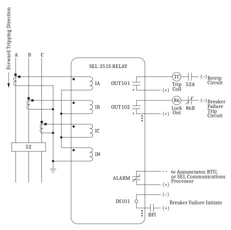
Current Channel IN does not need to be connected. Channel IN provides current  $I_N$  for the neutral-ground overcurrent elements. Separate from Channel IN, the residual ground overcurrent elements operate from the internally derived  $residual\ current\ I_G\ (I_G=3I_0=I_A+I_B+I_C).\ But\ in\ this\ residual\ connection\ example,\ the\ neutral\ ground\ and\ residual\ ground$ overcurrent elements operate the same because  $I_N = I_G$ .
