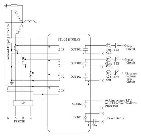
A core-balance current transformer is often referred to as a zero-sequence, ground fault, or window current transformer.
