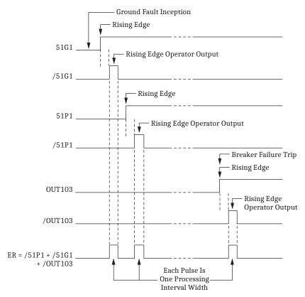
Figure F.1 Result of Rising Edge Operators on Individual Elements in Setting ER
