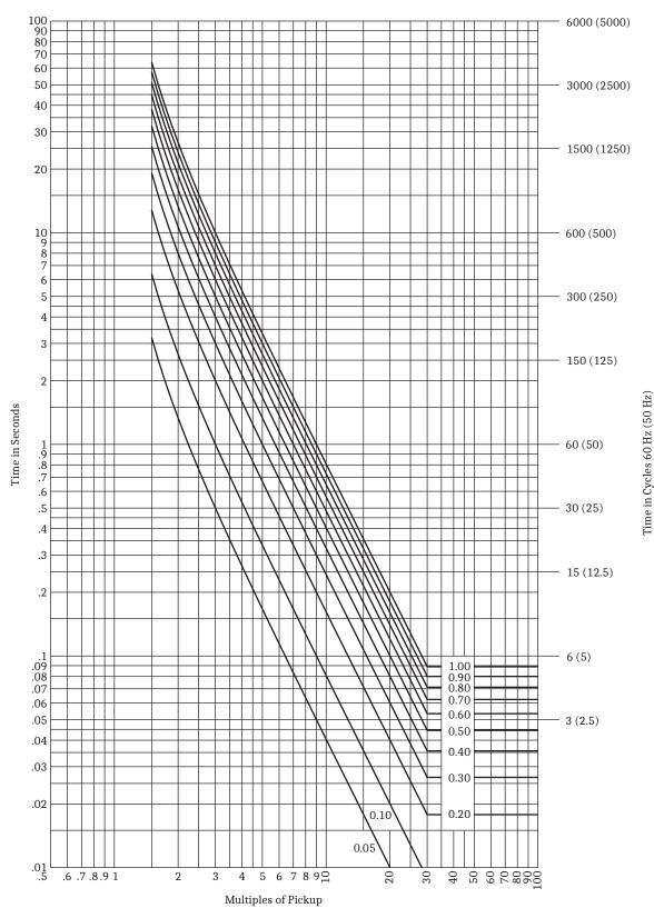
Figure 9.8 IEC Extremely Inverse (Class C) Curve (C3)
