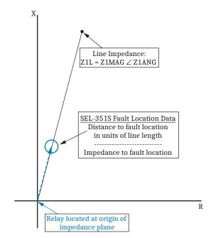
Figure R.1 Graphical Representation of SEL-351S Fault Location Data
