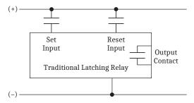
Figure 7.11 Traditional Latching Relay
