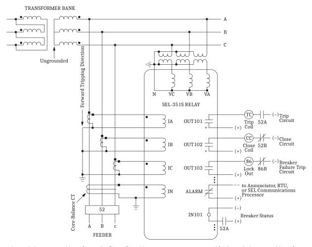
A core-balance current transformer is often referred to as a zero-sequence, ground fault, or window current transformer. Directional control for an ungrounded system is selected with setting ORDER = U (see Table 4.4-Table 4.6). Nondirectional sensitive earth fault (SEF) protection is also available.
