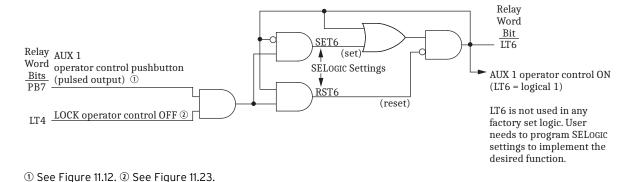
Figure 11.20 AUX 1 Operator Control Logic
