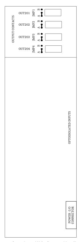
Figure 2.31 Jumper, Connector, and Major Component Locations on the SEL-351S Extra I/O Board With Four Standard Outputs (Extra I/O Board Option 4)
