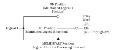
Figure 7.10 Remote Control Switches Drive Remote Bits RB1-RB32
