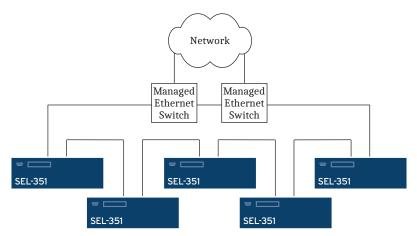
Figure 10.1 Self-Healing Ring Using Internal Ethernet Switch
