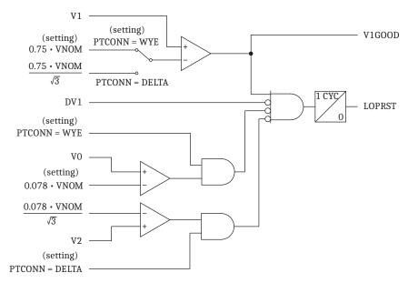
Figure 4.5 LOP Reset Logic (Relay Word Bit LOPRST)
