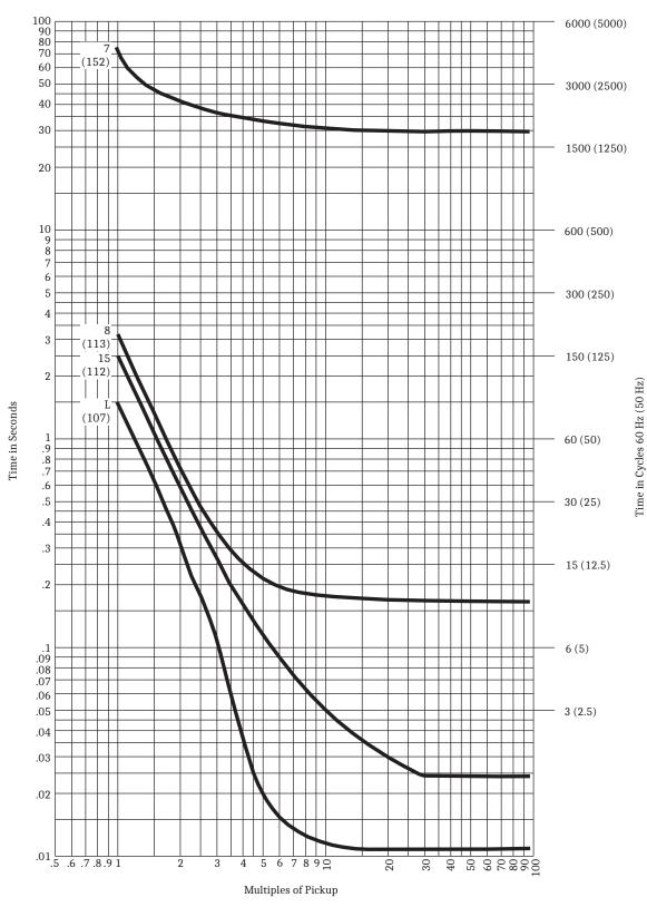
Figure 9.20 Recloser Control Response Curves L, 7, 8, and 15
