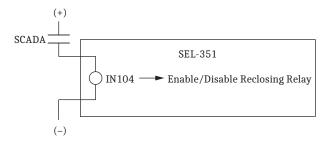
Figure 7.13 SCADA Contact Pulses Input IN104 to Enable/Disable Reclosing Relay
